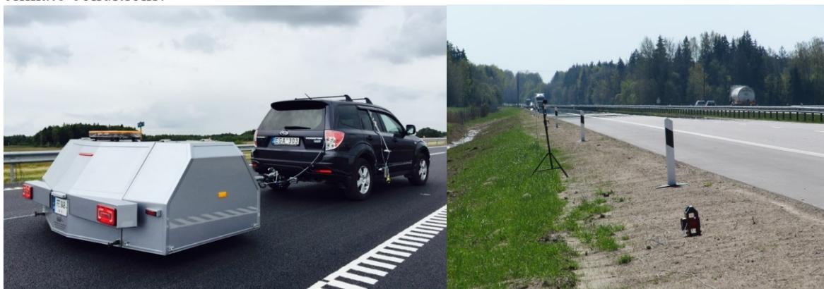
Figure 1 – Fragment from CPX (left) and SPB (right) noise level measurements
