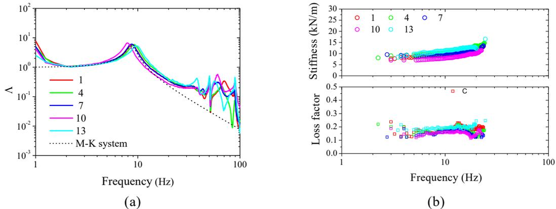
Figure 2 – (a) Measured and predicted transfer functions of the distributed dummy, (b) obtained dynamic stiffness and loss factor on the each locations
