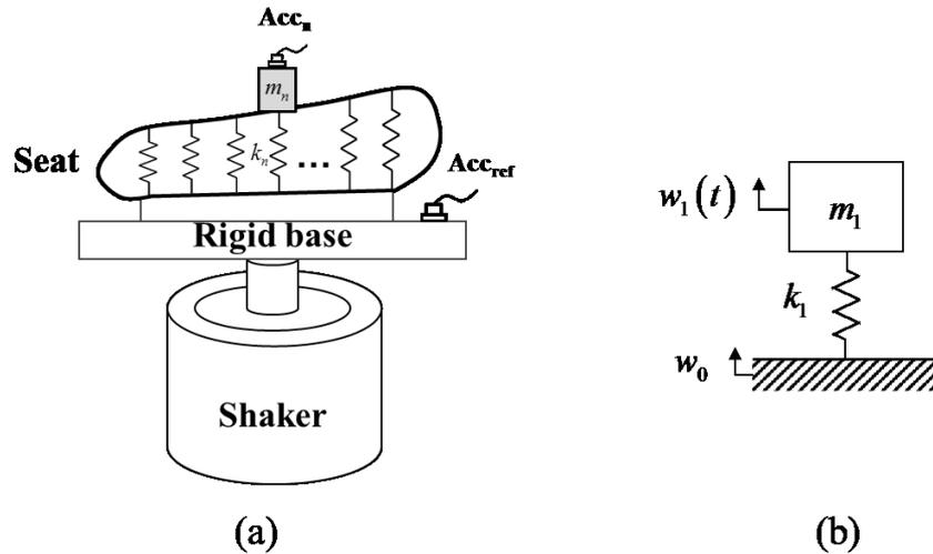
Figure 1 – (a) Distributed stiffness model of a seat supposed on a shaker and (b) mass-spring system.
