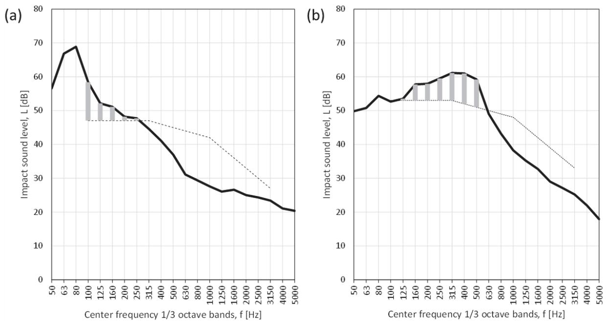
Figure 7: Mean impact sound spectrum (bold), shifted reference curve (dashed), and unfavourable deviations from the reference curve (grey columns) for (a) floating floor and (b) parquet on soft underlay on concrete slabs.
