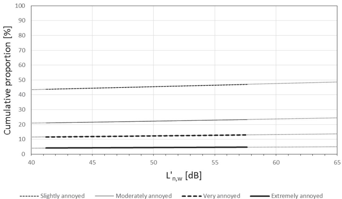
Figure 2: Cumulative proportion of annoyance for weighted normalized impact sound pressure level,  $L'_{n,w}$ .
