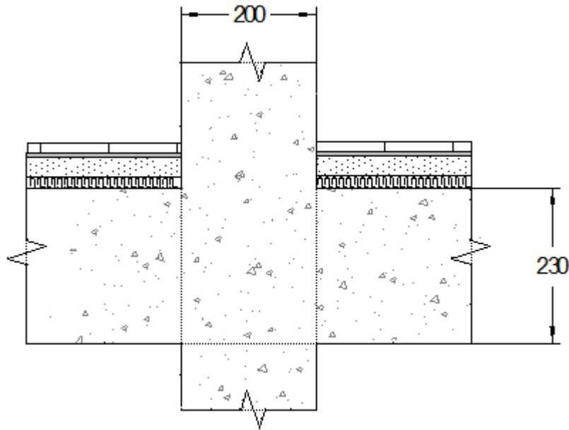
Figure 5: Example of load bearing construction combined with floating floor.
