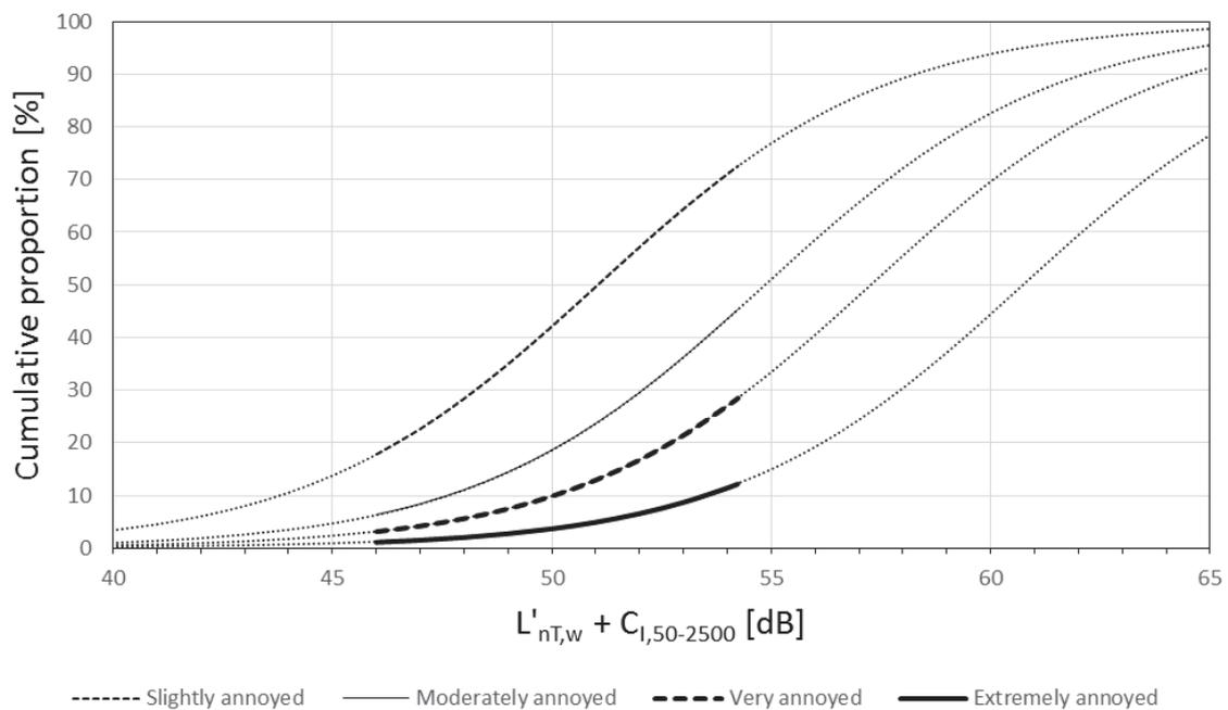
Figure 4: Cumulative proportion of annoyance for weighted standardized impact sound pressure level including spectrum adaptation term,  $L'_{nT,w} + C_{l,50-2500}$ . Bold sections of the lines represents 95 % confidence interval of the range of the measured data.
