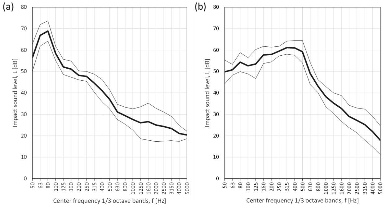
Figure 6: Mean impact sound spectrum (bold black), 95 % confidence interval (grey) for (a) floating floor and (b) parquet on soft underlay on concrete slabs.
