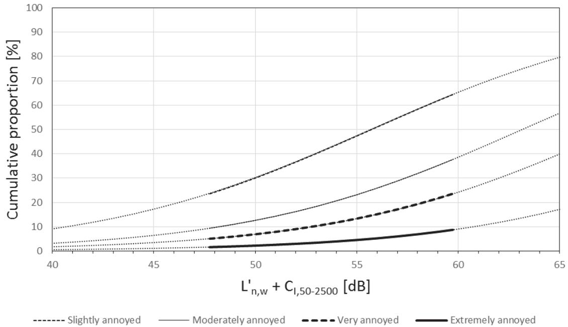
Figure 3: Cumulative proportion of annoyance for weighted normalized impact sound pressure level including spectrum adaptation term,  $L'_{n,w} + C_{l,50-2500}$ . Bold sections of the lines represents 95 % confidence interval of the range of the measured data.
