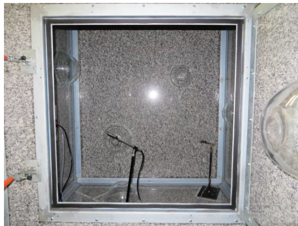
Figure 6 – The reverberation chamber with boundary diffusers.
