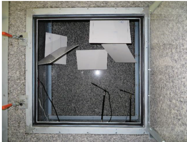
Figure 2 – The reverberation chamber with hanging panels diffusers.
