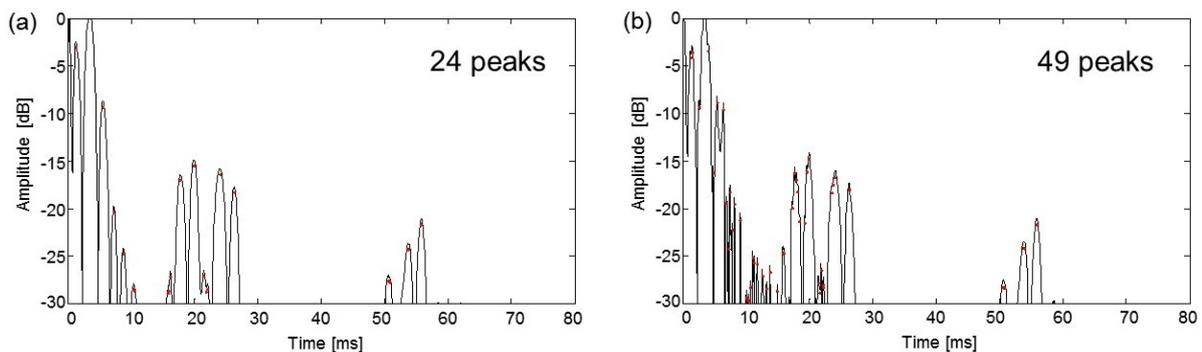
Figure 3 – Counting number of peaks ( $N_{p,early}$ ) (a) without a tree assuming as open field, and (b) with a tree on the ground in an anechoic chamber. The IRs were converted to full scale.
