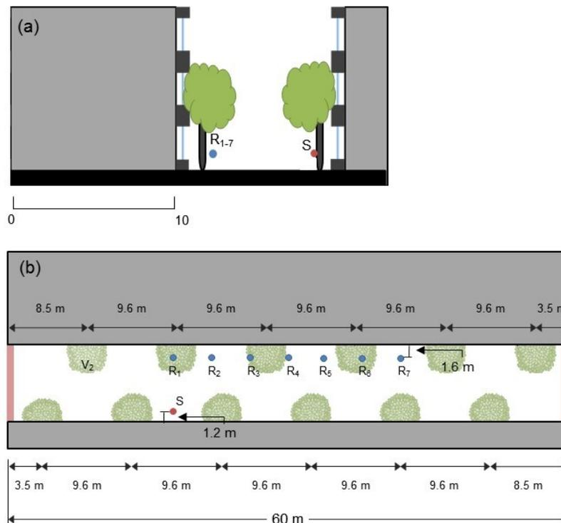
Figure 2 – (a) Section of street canyon with trees. (b) Plan view of roadside trees in the street canyon, and the source and receiver positions
