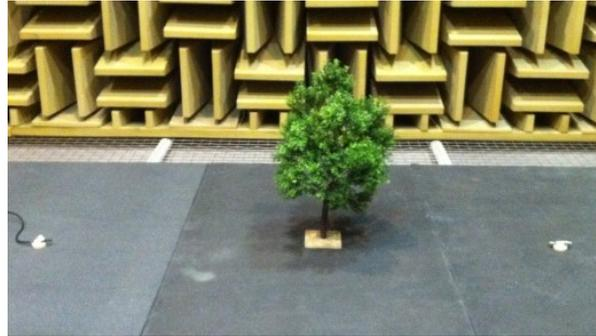
Figure 1 – A 1:10 scale model tree in an anechoic chamber
