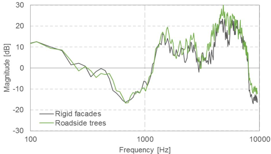
Figure 5 – Frequency responses of the case without a tree (Rigid façades, Grey line), and with roadside trees (Green line) in R1
