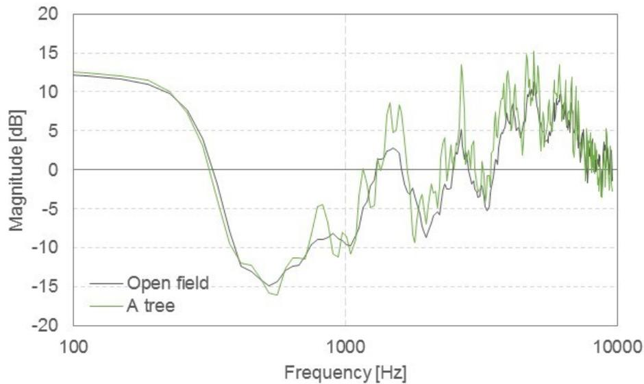
Figure 4 – Frequency responses of the case without a tree (Open field, Grey line), and with a tree (Green line)
