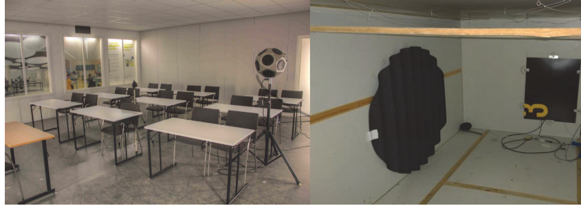
Figure 5: Left: The furnished room of the first example. Right: The scale model of the second example with the sinusoidal diffuser.
