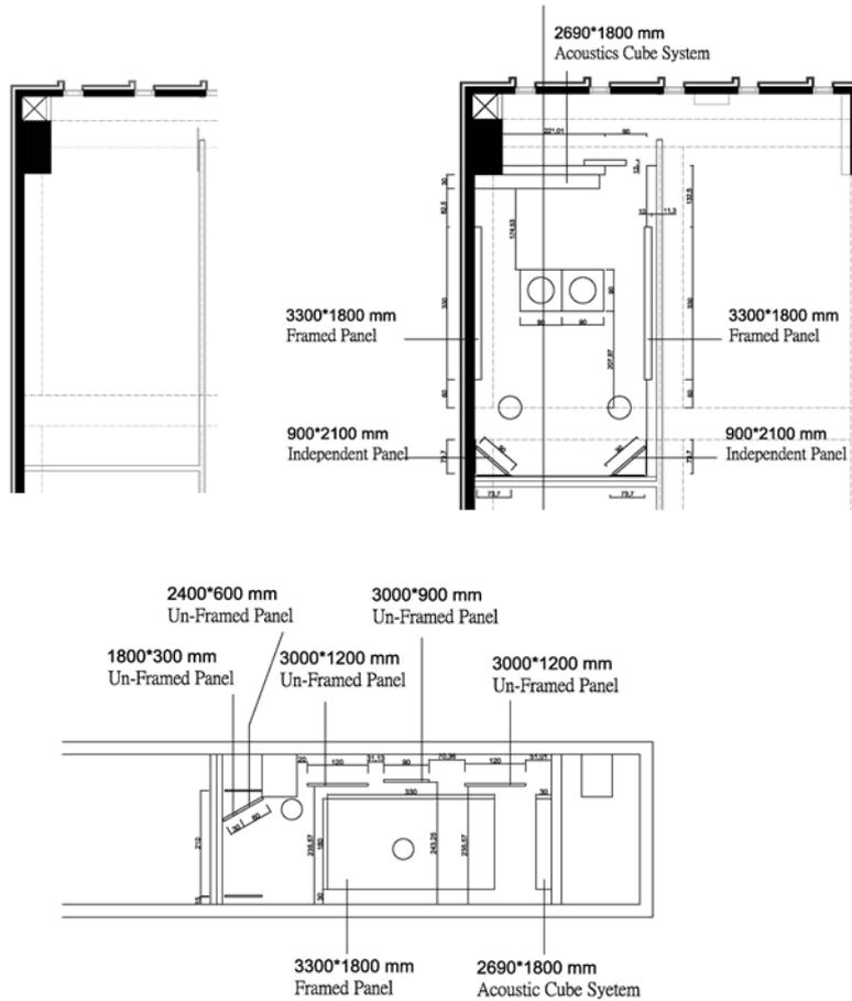
Figure 8 – Original space and distribution of ABS panel
