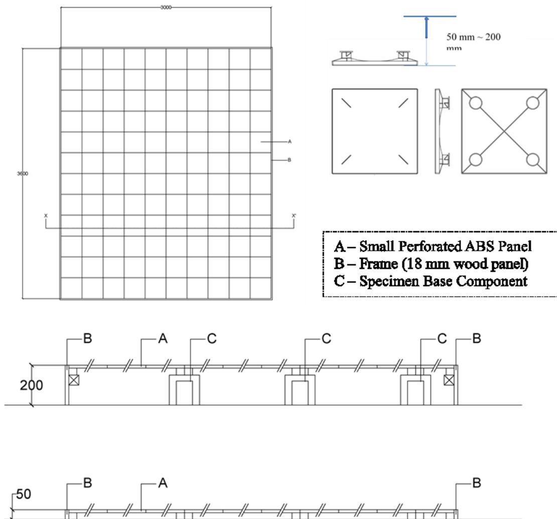
Figure 3 – Specimen setting
