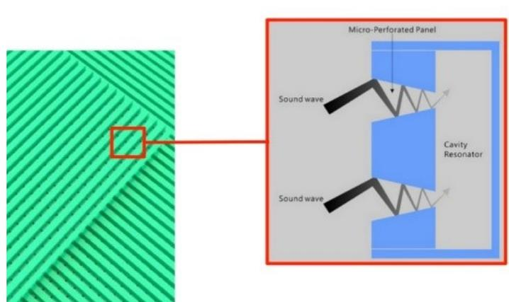
Figure 2 – Sound absorption of small perforated ABS panel
