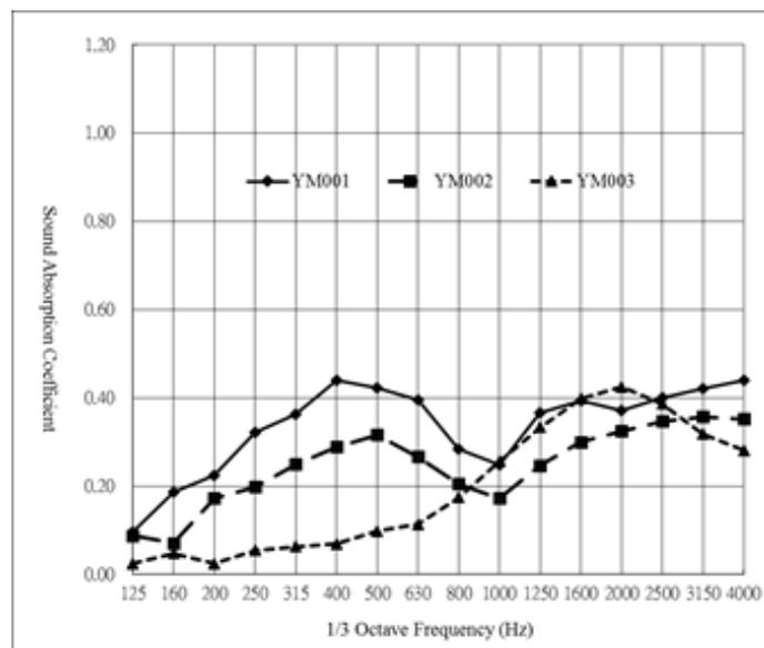
Figure 5 – Sound absorption of YM001, YM002, and YM003
