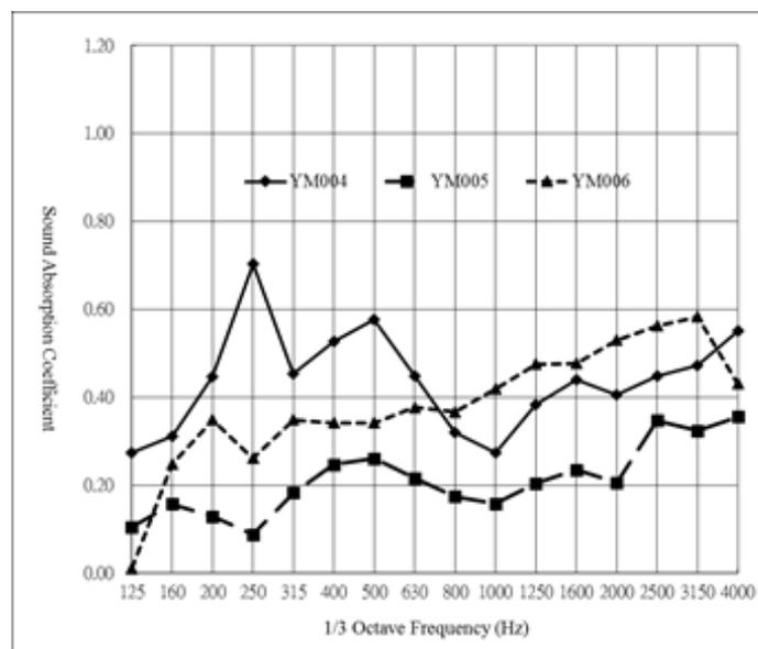
Figure 7 – Sound absorption of YM004, YM005, and YM006
