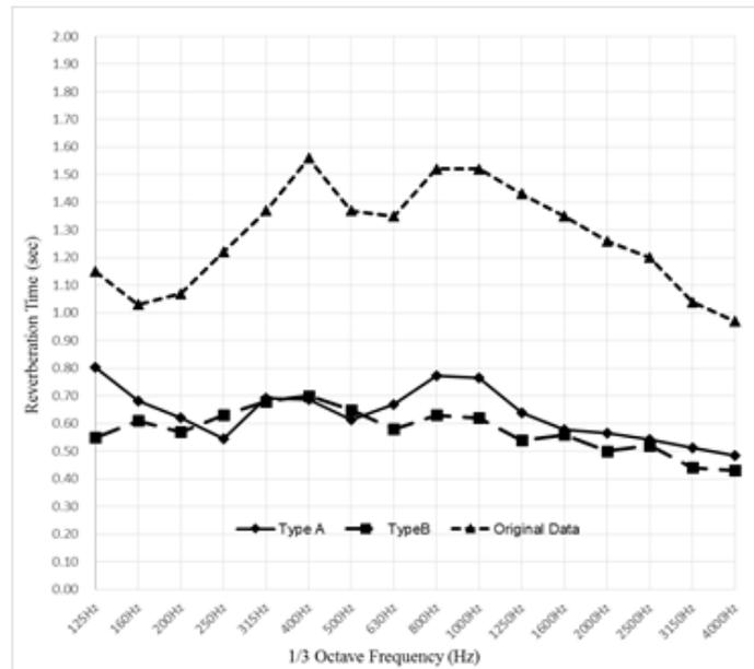
Figure 10 –Reverberation time of original space, calculation, and field measurement
