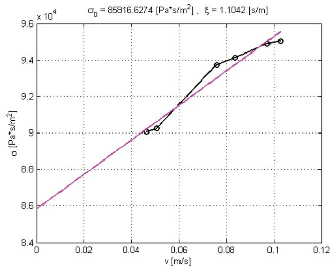
Figure 1: Flow resistivity measurements for a 1cm layer of Eurocarb ACF 1200
