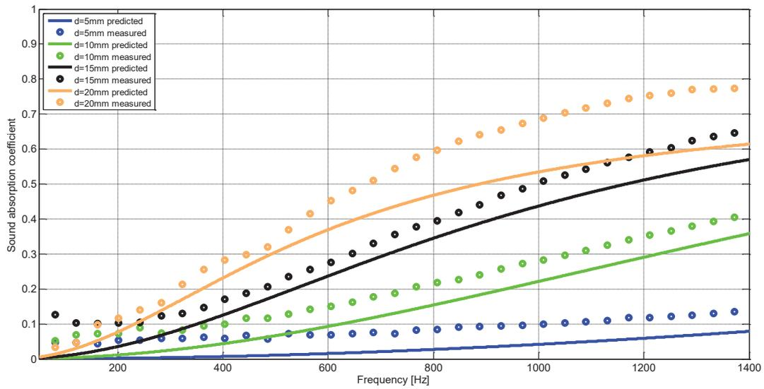
Figure 5: Comparison of the predicted vs. measured sound absorption coefficients for three different thicknesses of ACF 1200
