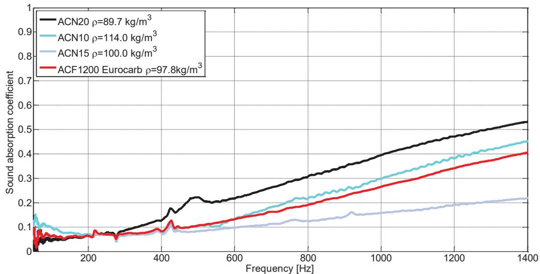
Figure 6: Comparison of the normal incidence sound absorption coefficients for different samples for a 1cm layer
