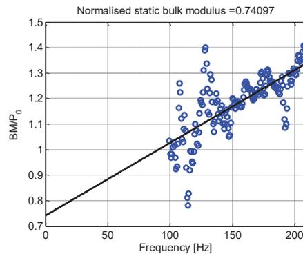
Figure 2: Bulk modulus at low frequency from two measurements of 4 and 8cm of Eurocarb ACF 1200
