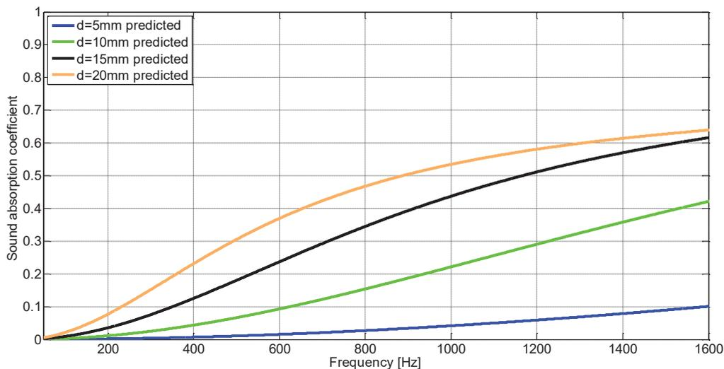
Figure 3: Normal incidence sound absorption coefficients of Eurocarb ACF1200 obtained by predictions
