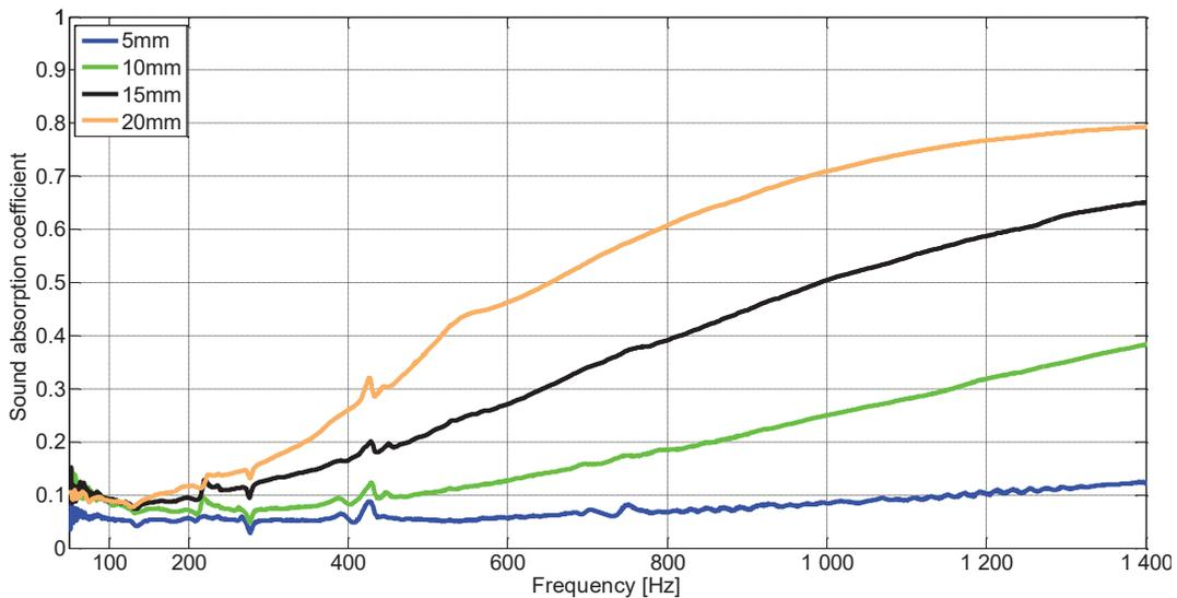
Figure 4: Sound absorption coefficients of the Eurocarb ACF1200
