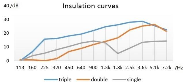
Figure 3 – Frequency attenuation (insulation curve after calculation).
