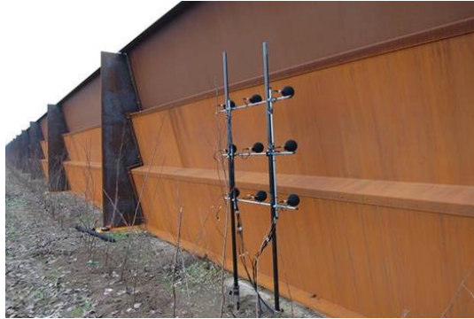
Figure 2 – Microphone array to determine the sound insulation
