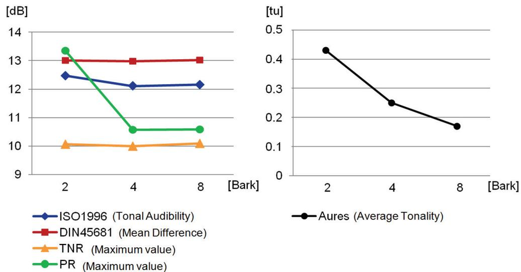
Figure 10 – Tonality indicators comparison,  $f_{\text{tone}} = 1200\text{ Hz}$ ,  $\Delta L_{\text{tone}} = 10\text{ dB}$
