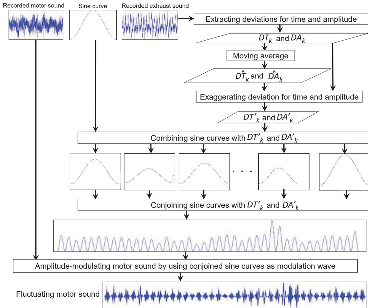
Figure 1 – Procedure for synthesizing fluctuating motor sound(16).
