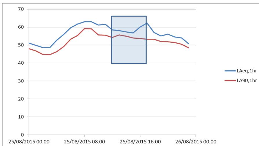
Figure 2 – Example of rain affected measurement data (periods of rainfall highlighted in blue box)
