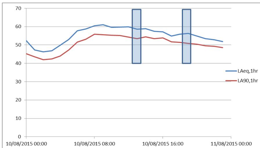
Figure 1 – Example of rain affected measurement data (periods of rainfall highlighted in blue box)
