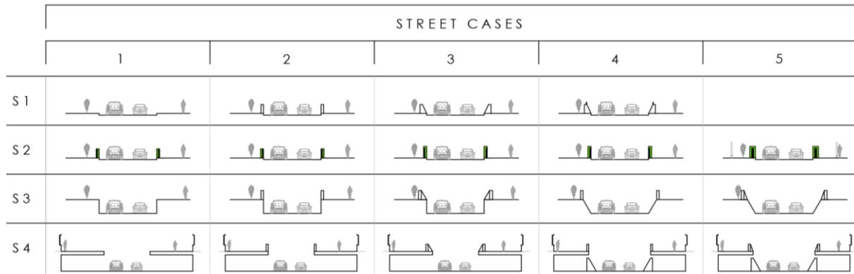
Figure 2–Street configuration cases (S). Sequences are distributed horizontally. S1 Low barrier shape. S2 Green absorption on low barrier. S3 Depressed road. S4 Two level street.
