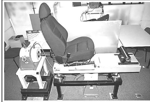
Figure 1 – Test bench with vibro-acoustic simulation
