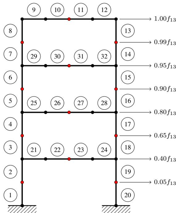
Figure 2: Considered frame structure with element numbering. The overall width of the frame is 4 m, while the height is 8 m.
