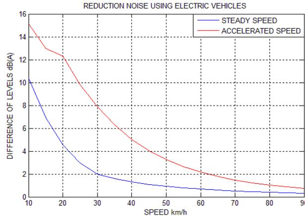
Figure 2 – Noise levels reduction depending on the driving conditions of a EVs flow
