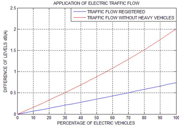
Figure 1 – Reduction of the noise levels in an urban environment due to the circulation of a EVs flow
