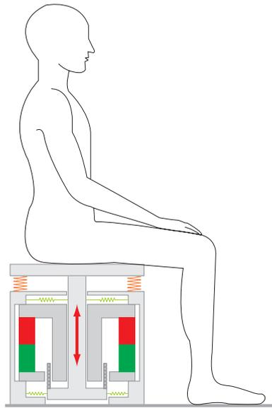
Figure 1 – Vibration chair with electrodynamic exciter.
