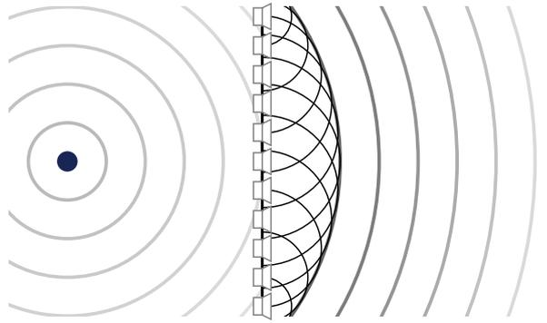
Figure 1: Concept of the wave field synthesis technology. An array of loudspeakers is individual driven so that the superposition of all sound waves radiated by the speakers generates the sound field of a virtual source.
