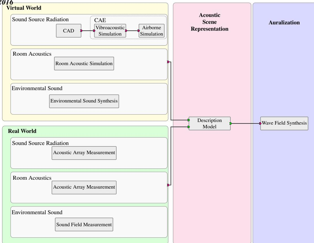
Figure 3: General concept of virtual acoustic signal acquisition. The representation of the acoustic scene is saved in a description model. The description model can be fed from simulation data (*Virtual World*) as well as from measurements and recordings (*Real World*).
