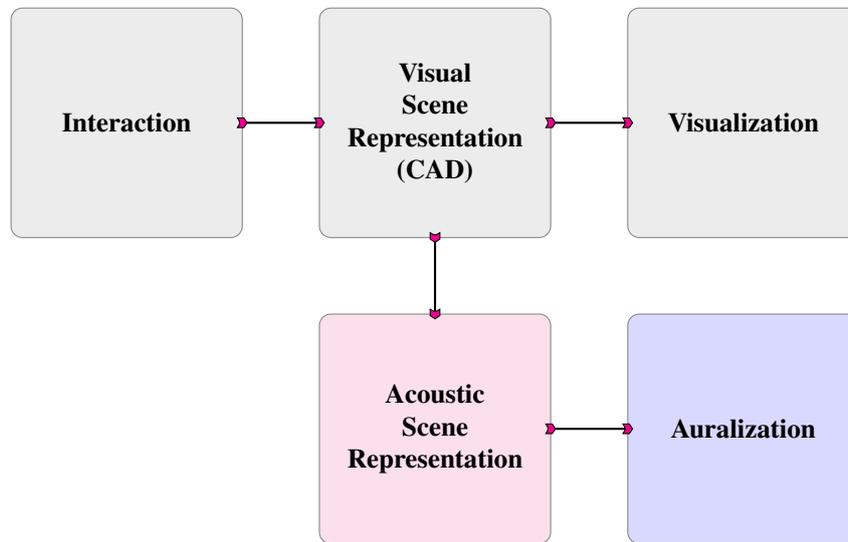
Figure 4: Detailed block diagram based on user interaction. A visual scene representation is interactively controlled, providing real-time (stereoscopic) visualization. As the visual scene is connected to the acoustic representation, user interaction directly controls the real-time auralization.
