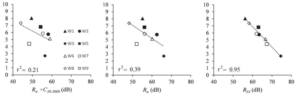
Figure 1 – Subjective variable as a function of  $R_w + C_{50-5000}$ ,  $R_w$ , and  $R_{S4}$ .
