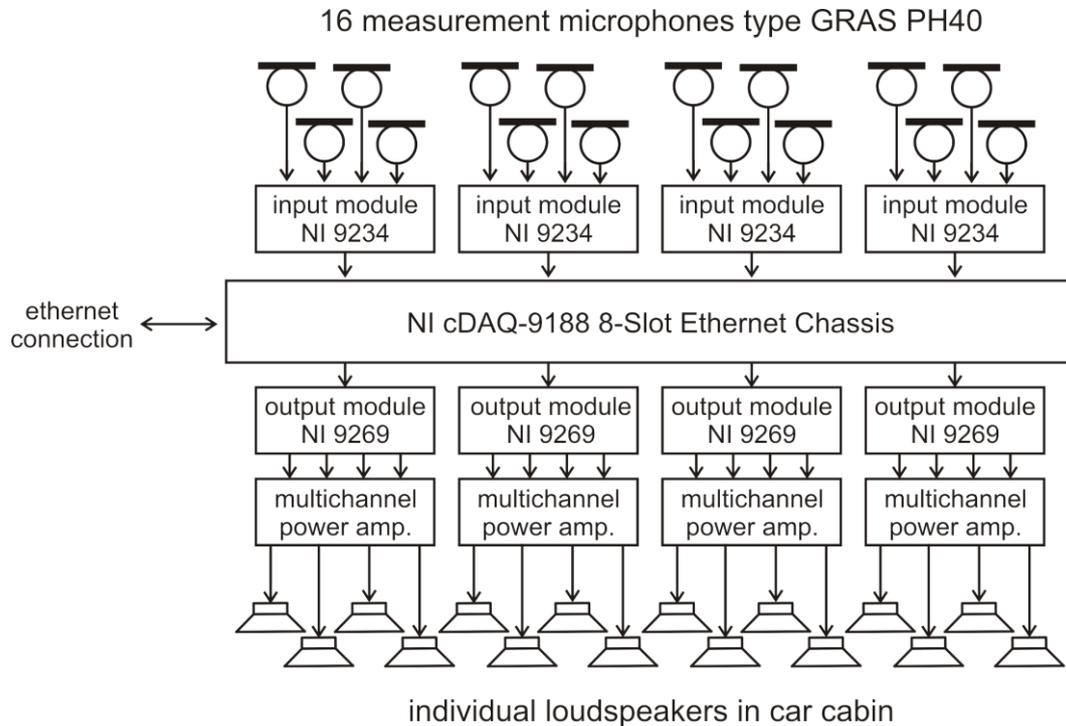
Figure 2 – A block diagram of the measurement system.
