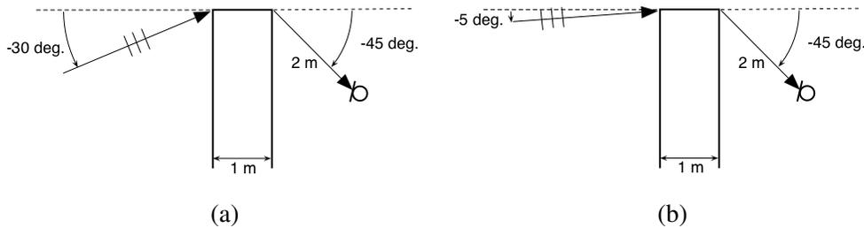
Figure 5 – Geometry for a flat-top noise barrier, with plane wave incidence angles of (a) -30 degrees, and (b) -5 degrees, relative to horizontal incidence.
