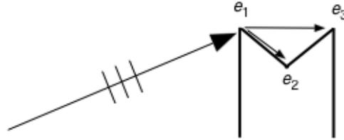
Figure 2 – A non-convex noise barrier top, with diffraction wave paths from edge  $e_1$  indicated.
