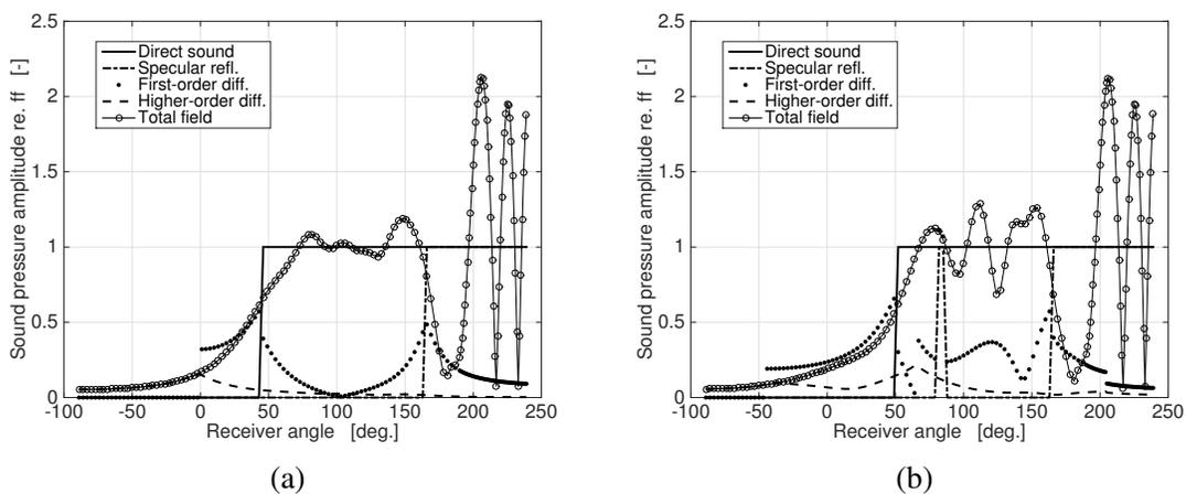
Figure 4 – The distribution of sound field components, as well as the total sound field, around the two noise barrier types in Figure 3. Results for the flat-top geometry are shown in (a), while (b) shows results for the triangular-top geometry. The sound pressure amplitude is normalized against the plane wave incidence, and is shown on a linear scale.
