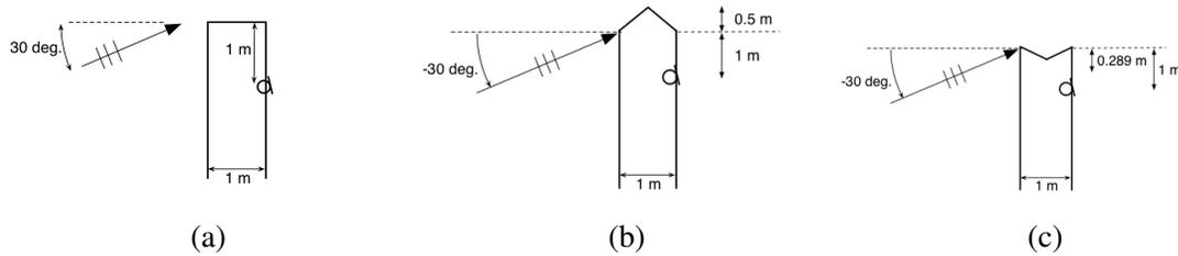
Figure 7 – A thick noise barrier with three different tops, with an incident plane wave as illustrated. A receiver is placed immediately at the surface of the noise barrier, as is also illustrated.
