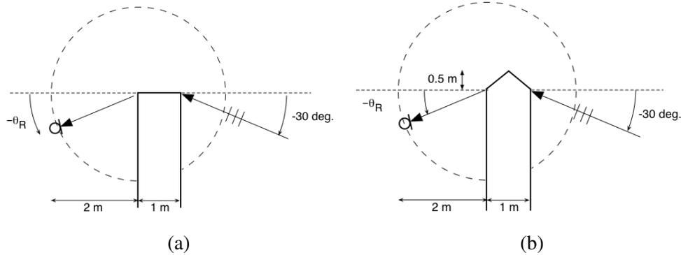
Figure 3 – Geometry of two noise barriers, with (a) Flat top, (b) Triangular top.
