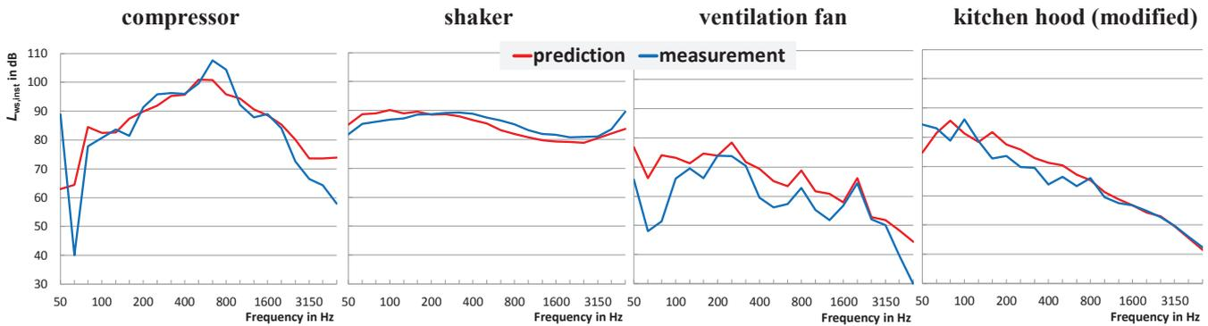
Figure 3 – Installed structure-borne sound power level  $L_{Ws,inst}$  on a receiving structure frequency for different sources; comparison of prediction according to [2] (red) and measurements with the reception plate method (blue)
