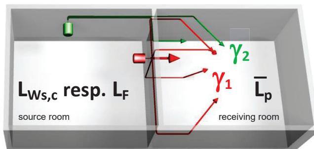
Figure 1 – Relevant sound transmission paths for the measurement of the transfer index  $\gamma$ . Type 1: Source connection on the separating wall (red). Type 2: Source connection on a flanking element (green)
