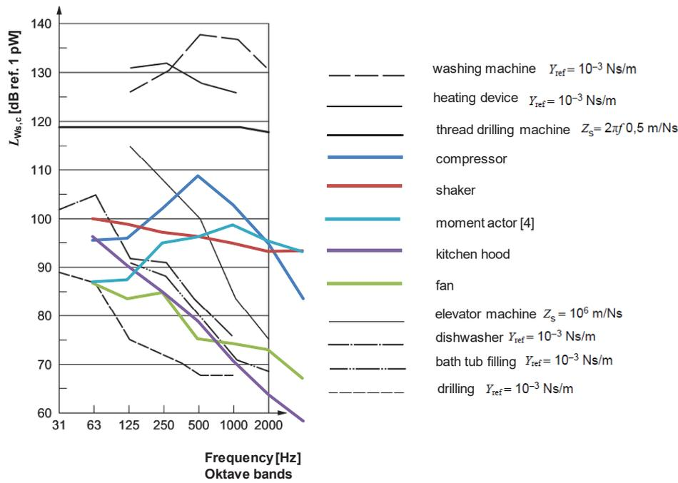
Figure 2 – Characteristic structure-borne sound power level  $L_{Ws,c}$  according to [2] and for different sources characterised by TSM
