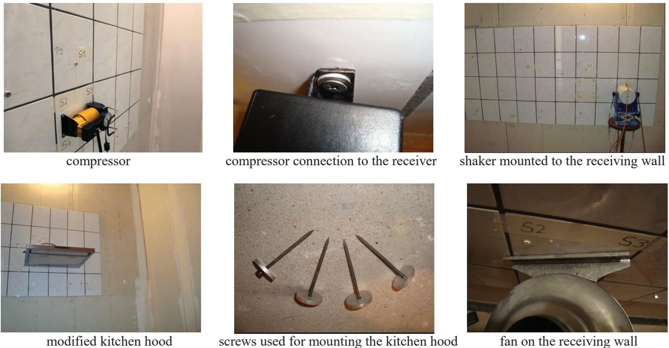
Figure 4 – Common structure-borne sound sources in the source room of the light-weight test facility at PTB Braunschweig
