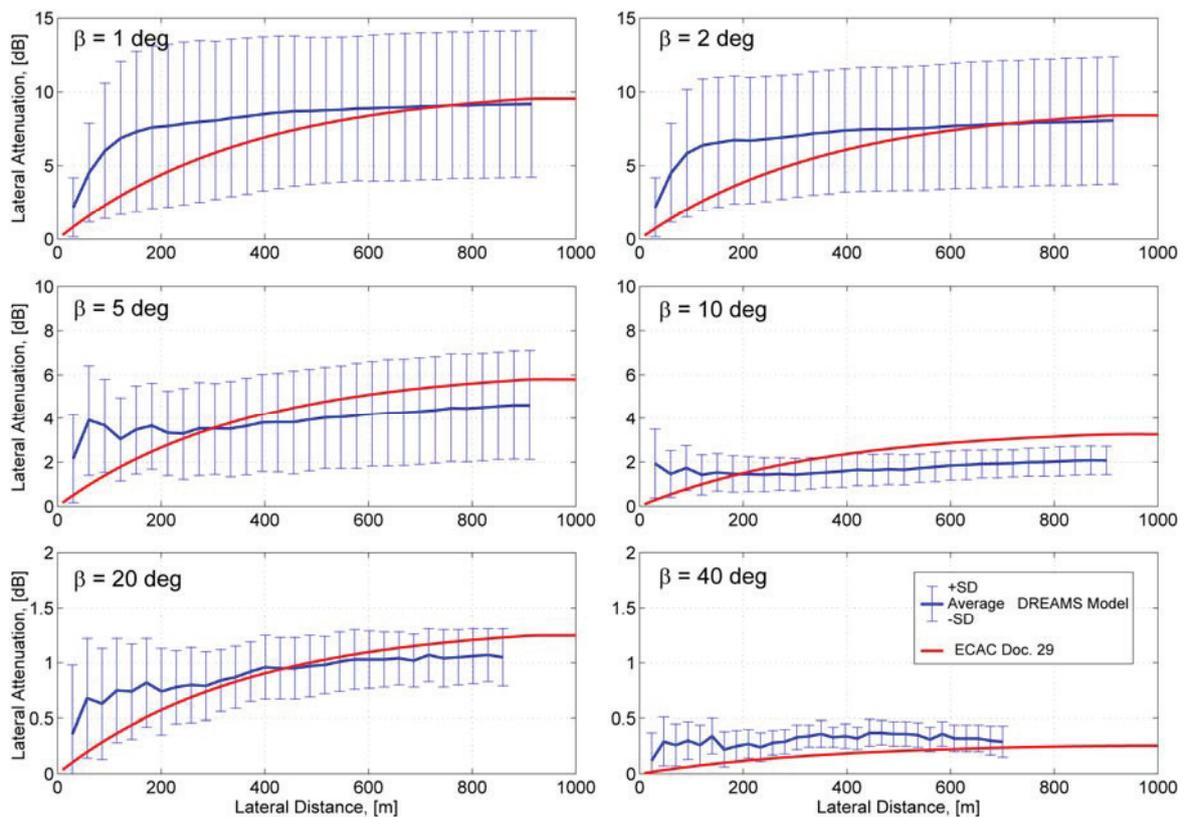
Figure 2 – Comparison of lateral attenuation predicted by DREAMS' model and ECAC Doc.29
