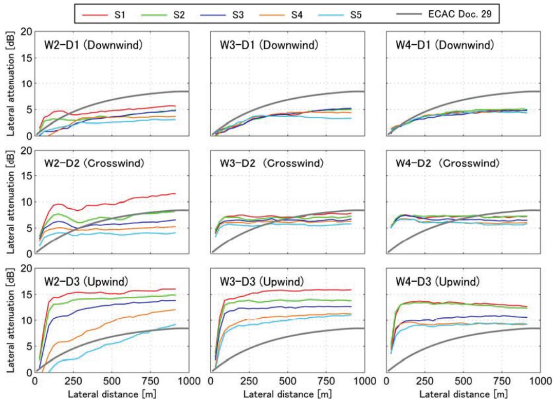
Figure 3 – Difference of lateral attenuation due to meteorological conditions ( $\beta=2$  deg)
