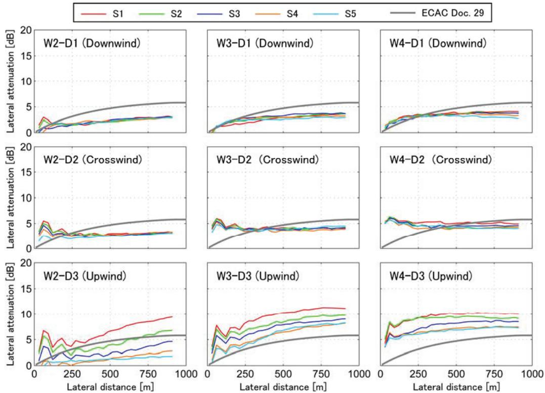
Figure 4 - Difference of lateral attenuation due to meteorological conditions ( $\beta=5$  deg)
