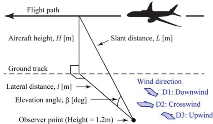
Figure 1 – Definitions of geometric parameters
