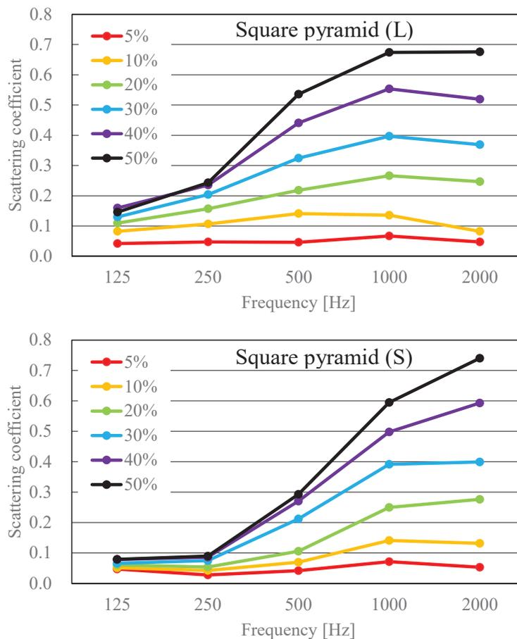
Figure 8– Frequency characteristics of estimated scattering coefficients of large and small diffusers in each area ratio of diffusers
