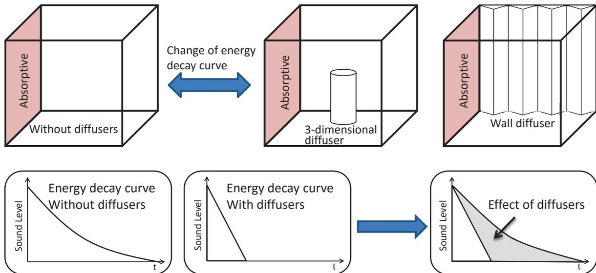
Figure 1 – Basic idea for measuring scattering capability of diffusers
