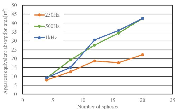
Figure 11– Estimated apparent equivalent absorption area vs. number of spheres
