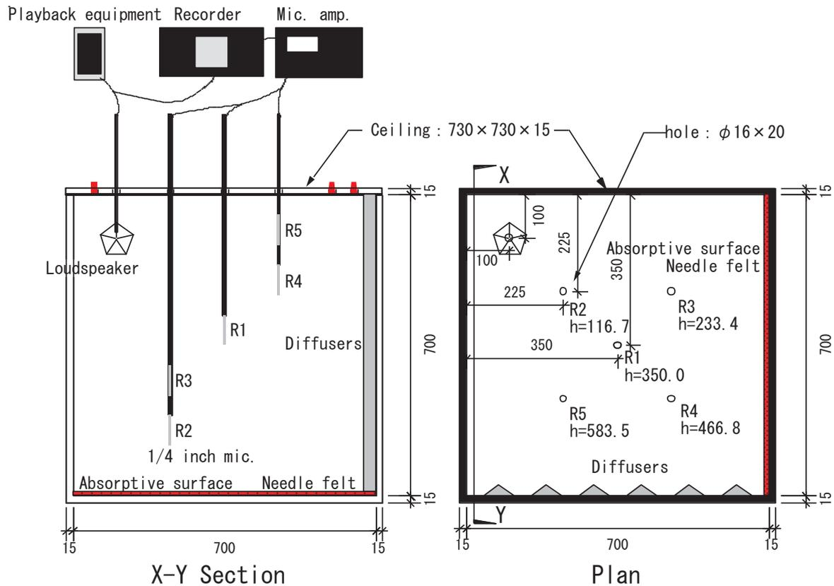
Figure 6 – Block diagram of 1/10 scale model experiment, and arrangement of a sound source and receiving points R1 – R5.
