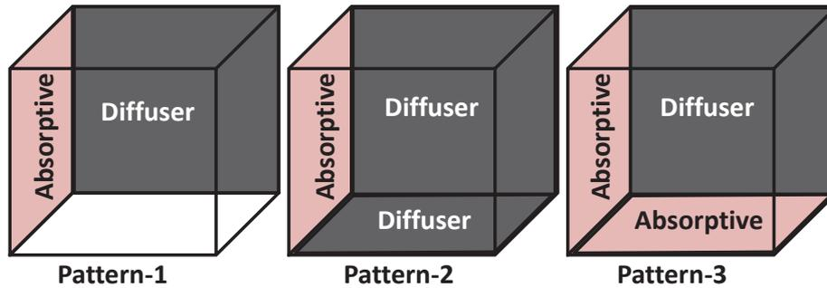
Figure 2 – Patterns of absorption-diffusion treatment of walls
