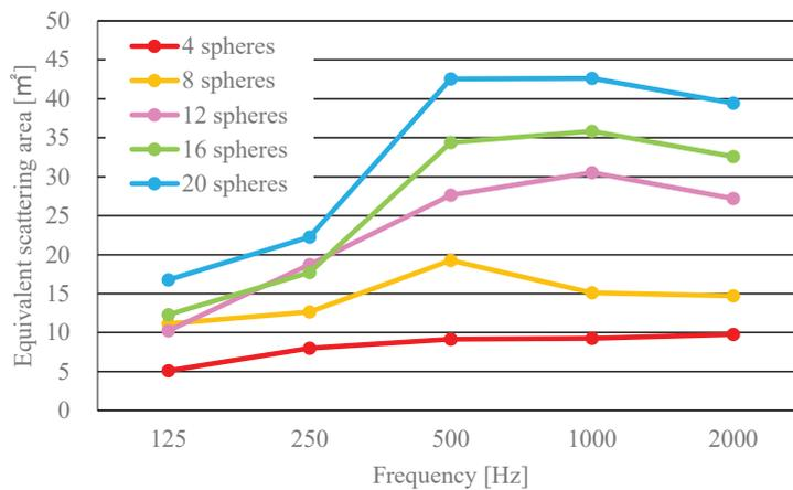
Figure 10– Frequency characteristics of estimated apparent equivalent absorption area
