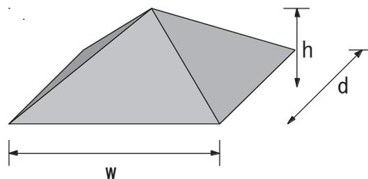
Figure 7 – Configuration of a diffuser used in the experiment
