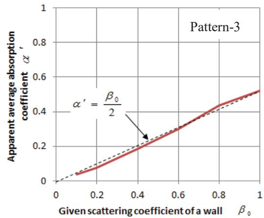
Figure 5 – Apparent average absorption coefficients vs. given scattering coefficient of a wall
