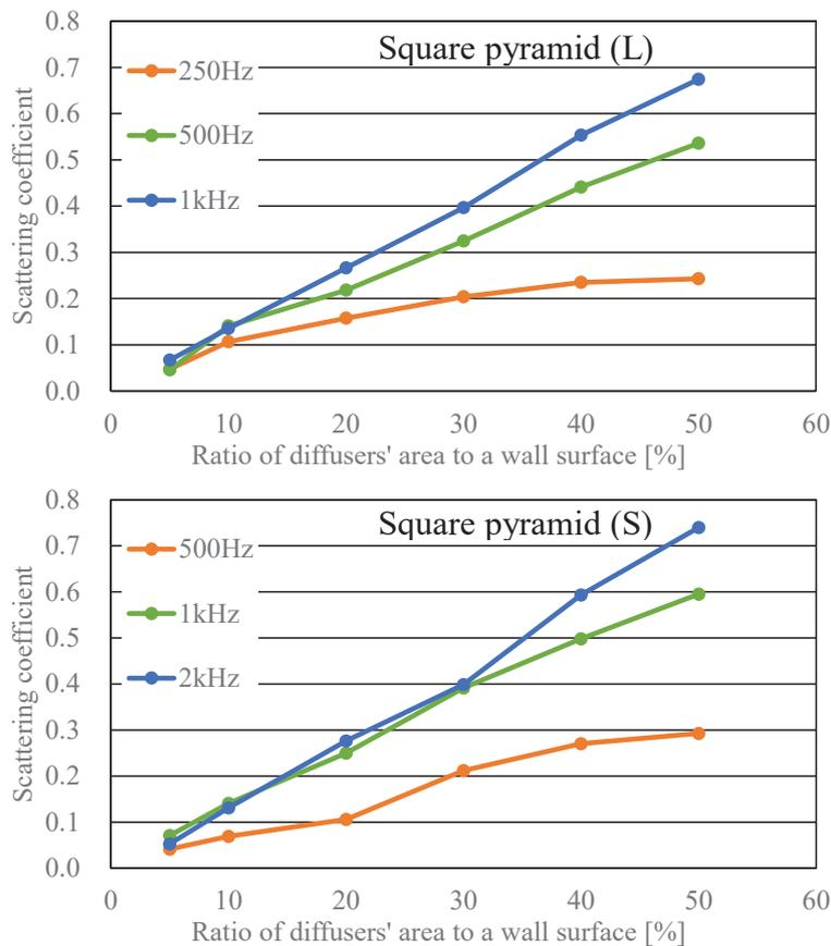
Figure 9– Estimated scattering coefficients vs. area ratio of diffusers to a wall surface
