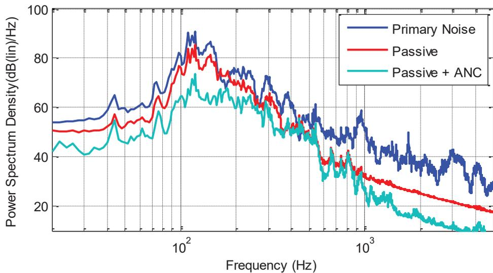
Figure 7 - Performances of the Active Labyrinth configuration
