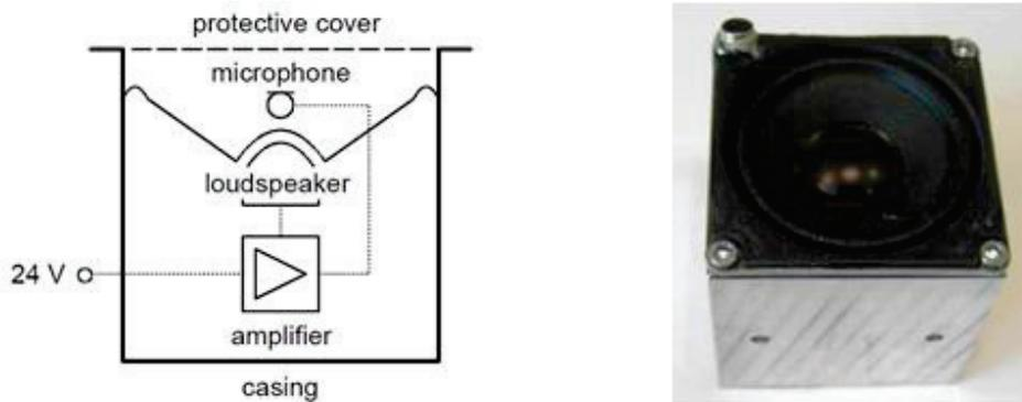
Figure 4 - ASCa module schematics (left) and picture (right) designed by the Fraunhofer Institute for Building Physics
