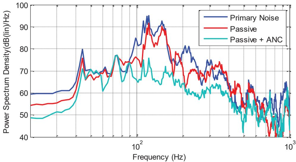
Figure 6 - Performances of the Active Window configuration
