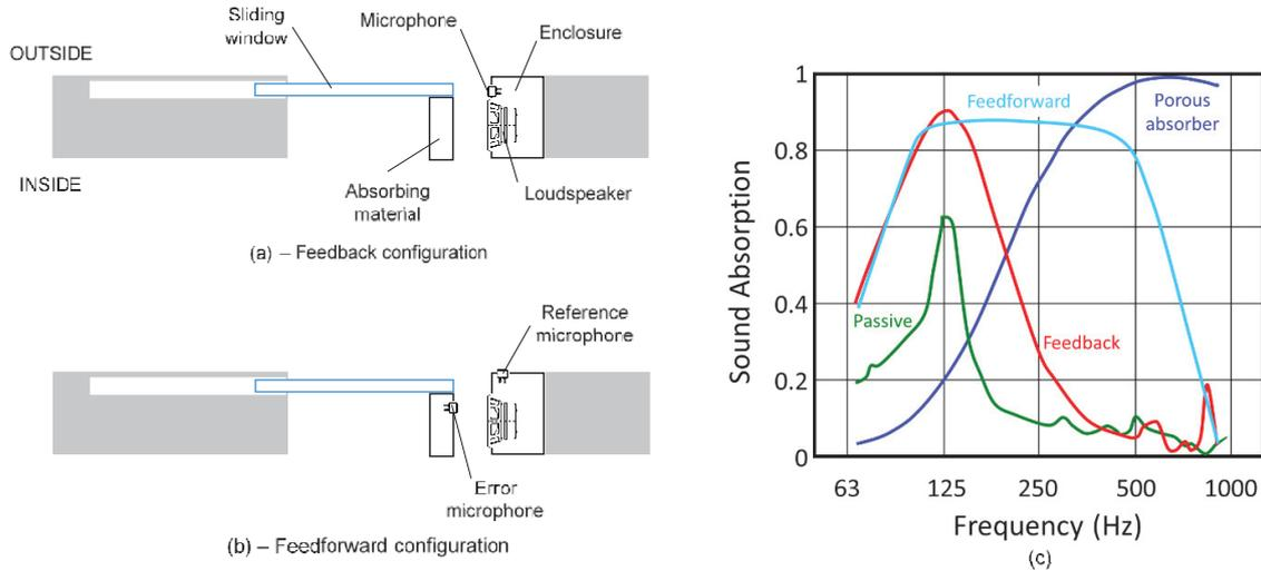
Figure 2 - Active Window feedback (a) and feedforward (b) configurations. Typical sound absorption (c)
