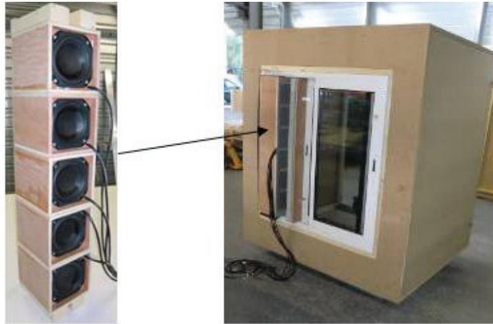
Figure 5 - Picture of the test bench with Active Window configuration
