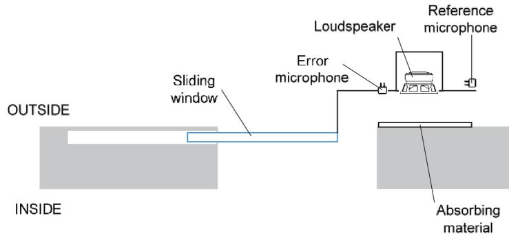
Figure 3 - Active Labyrinth feedforward configuration
