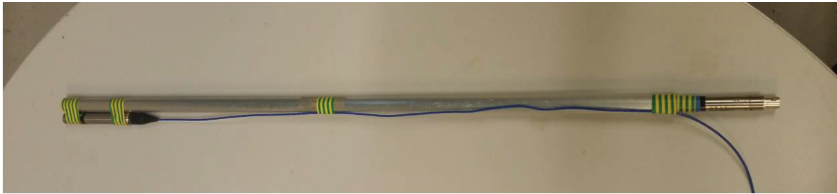
Figure 1 – Passive acoustic thermometer consisting of two microphones and an aluminum tube. The internal microphone stops the pipe to detect its resonances and an external microphone is used to remove artifacts in the ambient noise spectrum.
