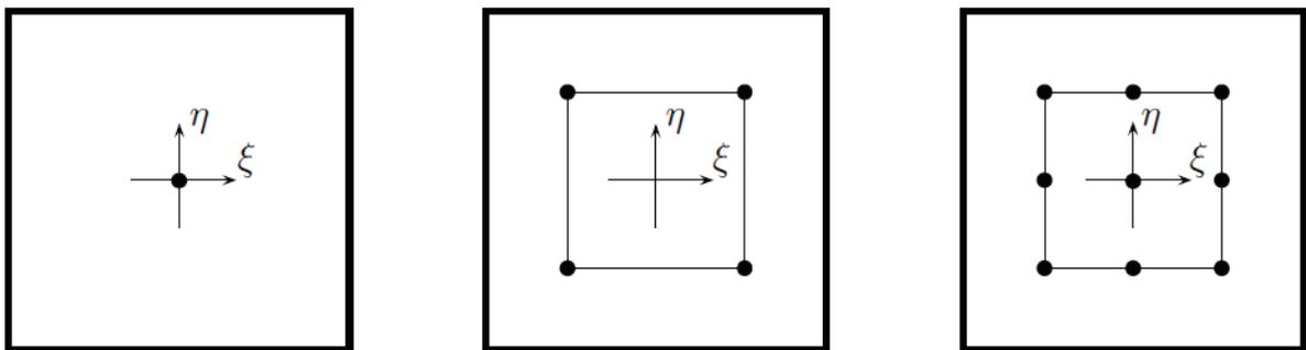
Figure 3: Discontinuous elements (constant, linear and quadratic)
