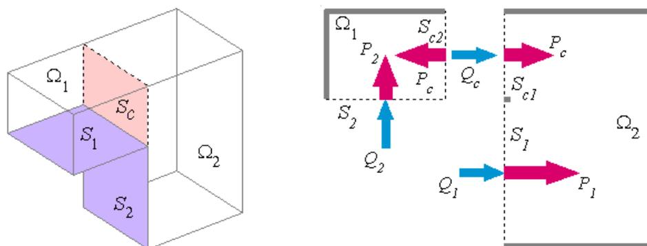
Figure 2 – Modelling of impedance of an L-shaped cavity
