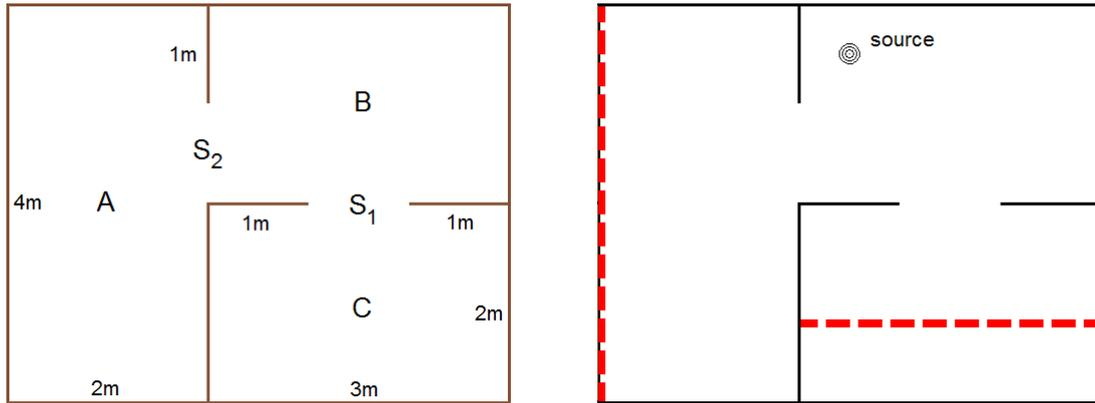
Figure 6 – The acoustical space. Left: geometry; right: source and response positions.
