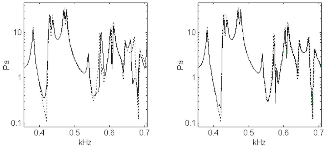
Figure 3 – Sound pressure response by patch coupling (full line) and direct solution (dotted line). Left: mean patch size / mean wavelength = 0.3; 10,000 modes. Right: mean patch size / mean wavelength = 0.15; 316,000 modes.
