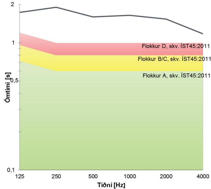
Figure 1 – Measured reverberation time in stairway, and quality classification (ÍST45)
