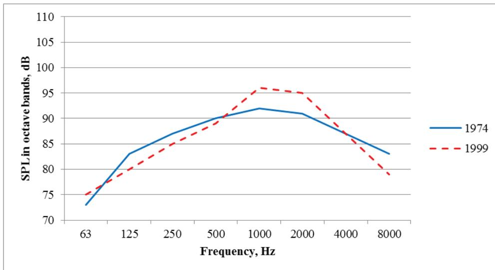
Figure 4: Comparison of frequency spectra of vehicle pass-by measurements for light vehicles at 50 km/h made in 1974 and 1999. Data adapted from Sandberg, 2001 [8].
