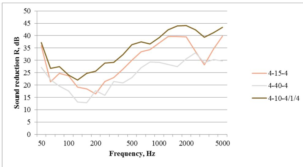
Figure 6: Sound reduction of the three window types used in the calculations.
