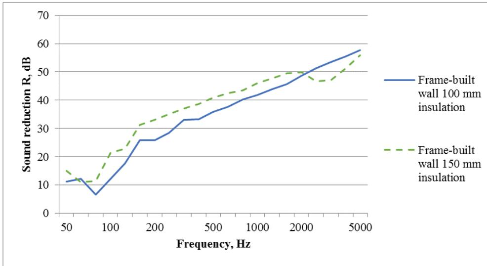
Figure 7: Sound reduction of the two wall types used in the calculations.
