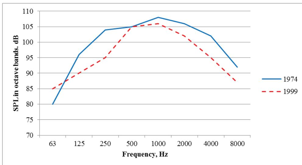
Figure 5: Comparison of frequency spectra of vehicle pass-by measurements for heavy trucks at 70 km/h made in 1974 and 1999. Data adapted from Sandberg, 2001 [8].
