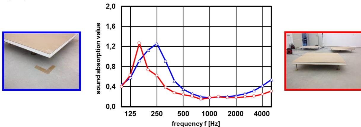
Figure 9 – sound absorption value by covered front and reverse site
