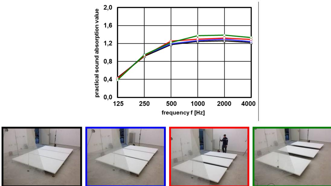
Figure 5 – practical sound absorption value for different distances between the canopies (canopy 2.4 x 1.2 m)
