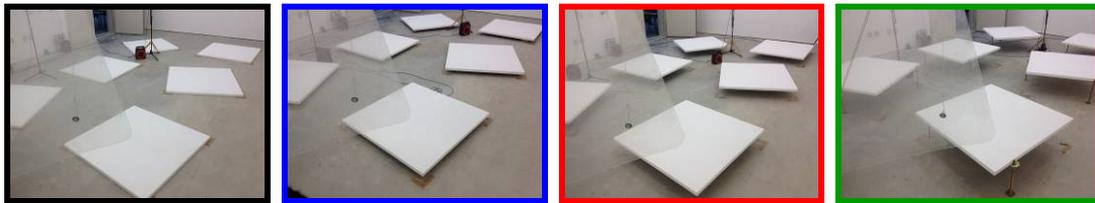
Figure 2 – practical sound absorption value for different suspension heights (canopy 1.2 x 1.2 m)
