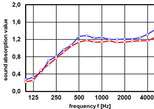
Figure 7 – sound absorption of canopy E40 vs. rear side covered with 10 mm MDF tile (E200)
