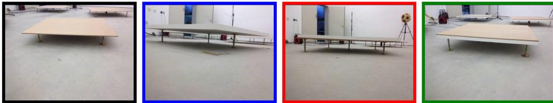
Figure 6 – practical sound absorption value of the full canopy, only the front side and only the reverse side
