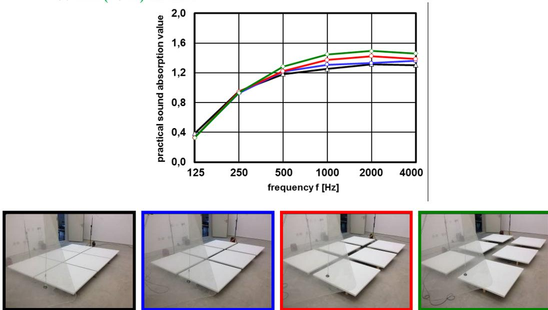
Figure 4 – practical sound absorption value for different distances between the canopies (canopy 1.2 x 1.2 m)
