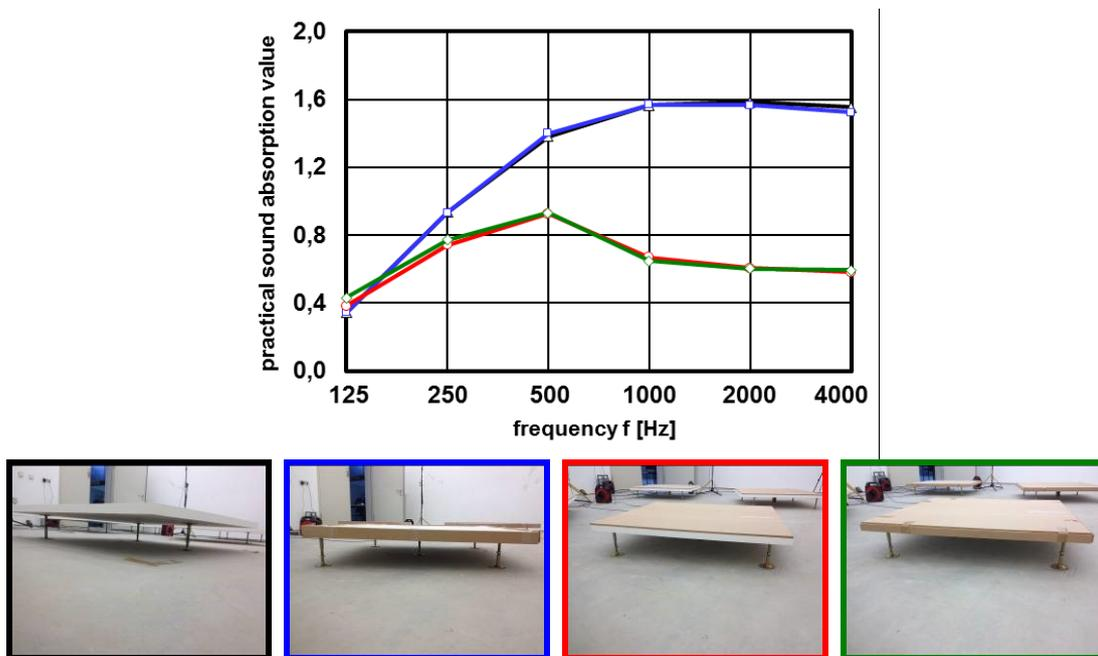
Figure 8 – practical sound absorption value to determine the edge effect
