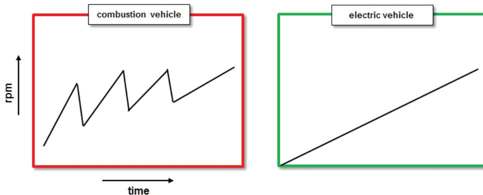
Figure 3 – Schematic representation of the rpm for a traffic light start maneuver. Left: combustion engine; right: electric engine
