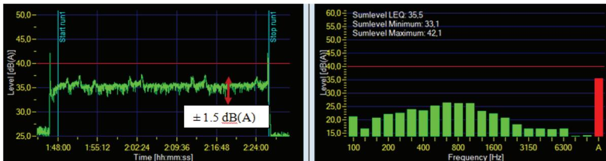
Figure 13. Sound power and frequency spectrum for the capillary insert length 17 mm.
