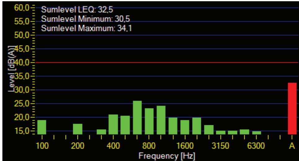
Figure 10. Solo compressor sound power level and frequency spectrum.
