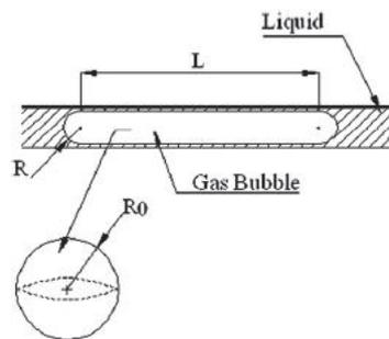
Figure 4. Deformation of the bubble (7)
