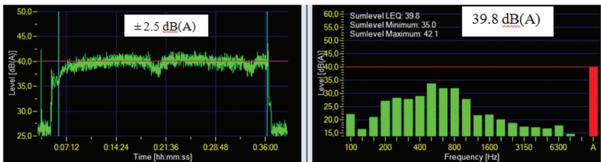
Figure 9. Sound power and frequency spectrum for the capillary insert length 7 mm.
