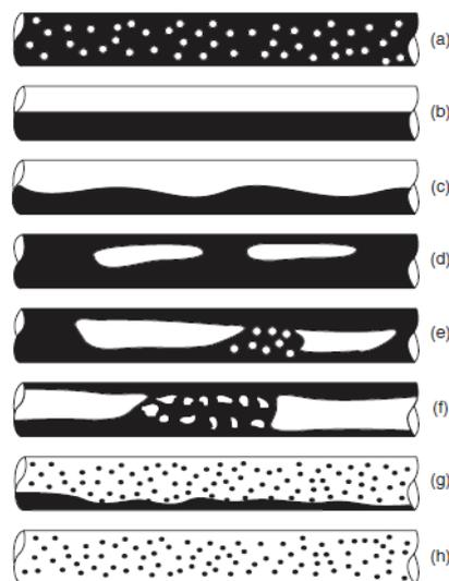
Figure 3. Flow patterns in horizontal pipes: (a) bubbly flow, (b) stratified flow, (c) wavy flow, (d) plug flow, (e) slug flow, (f) froth flow, (g) annular mist flow, (h) mist flow (3).
