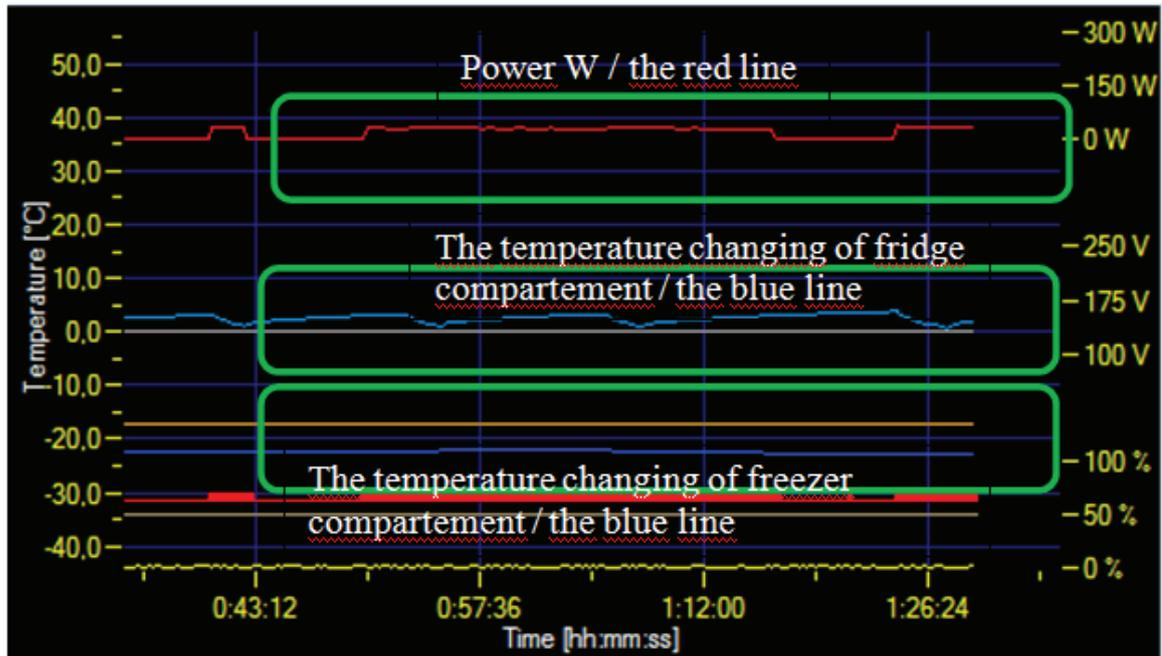
Figure 8. The cyclic temperature and electric power of the refrigerator.
