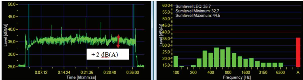
Figure 12. Sound power and frequency spectrum for the capillary insert length 15 mm.
