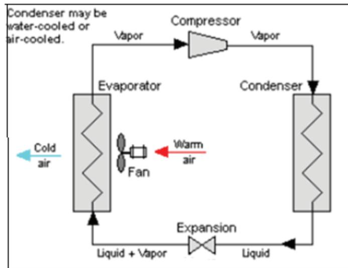
Figure 2. A schematic view of the refrigeration system (2).
