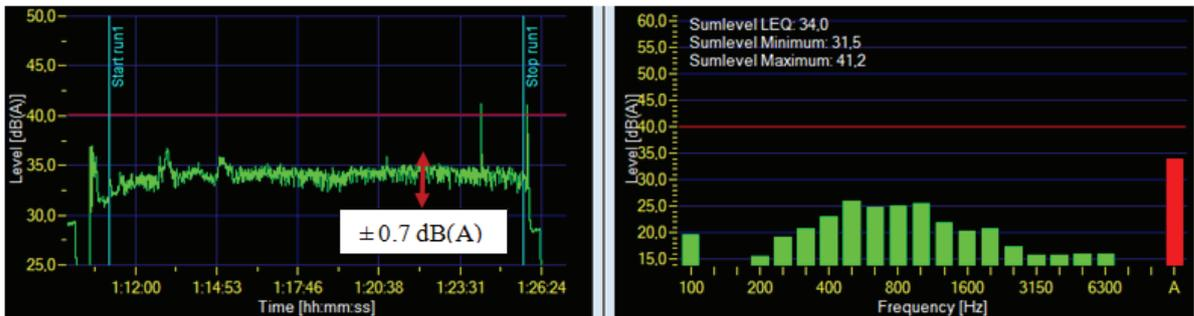
Figure 14. Sound power and frequency spectrum for the capillary insert length 20 mm.
