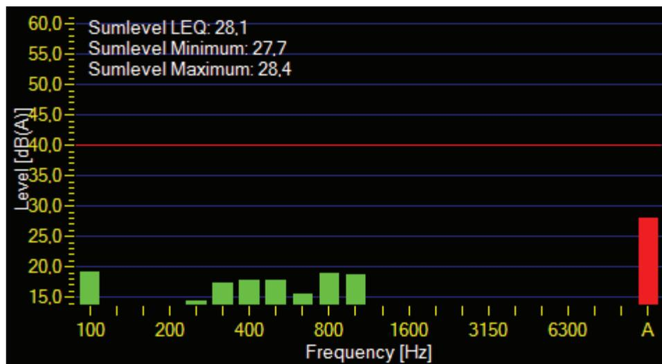
Figure 11. Solo fan sound power level and frequency spectrum.
