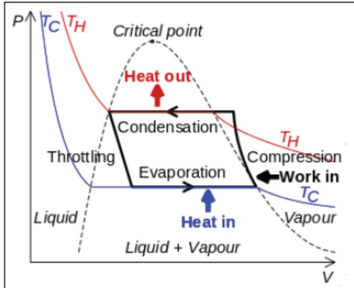
Figure 1. A fictitious pressure-volume diagram for a typical refrigeration cycle (2).
