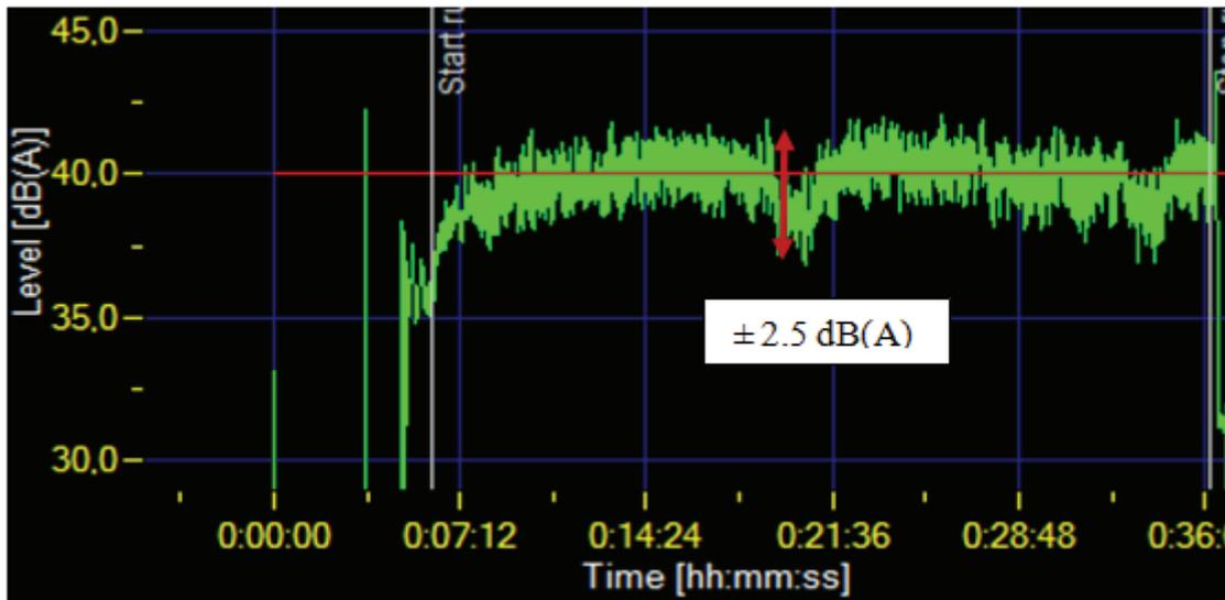
Figure 7. Sound power level variation of the refrigerator.
