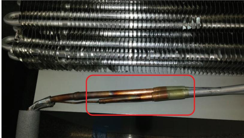
Figure 5. Capillary tube inlet of the evaporator.
