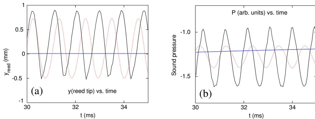
Figure 3. Effect of reed damping. (a) Left: Position of the reed tip as a function of time. (b) Right: Sound pressure as a function of time. Black curves:  $R = 450$ ; Red curves:  $R = 250$ ; Blue curves:  $R = 0$ . There was no oscillation with  $R = 0$ .
