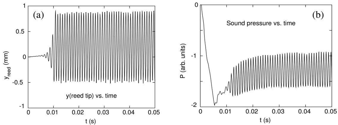
Figure 1. (a) Left: Position of the reed tip as a function of time.  $y_{\text{reed}} = 0$  corresponds to an undisplaced reed tip. (b) Right: Sound pressure outside the instrument as a function of time. The air speed in the mouthpiece was 5 m/s and the dimensionless lip-reed damping was  $R = 450$  (to be compared with other results below).
