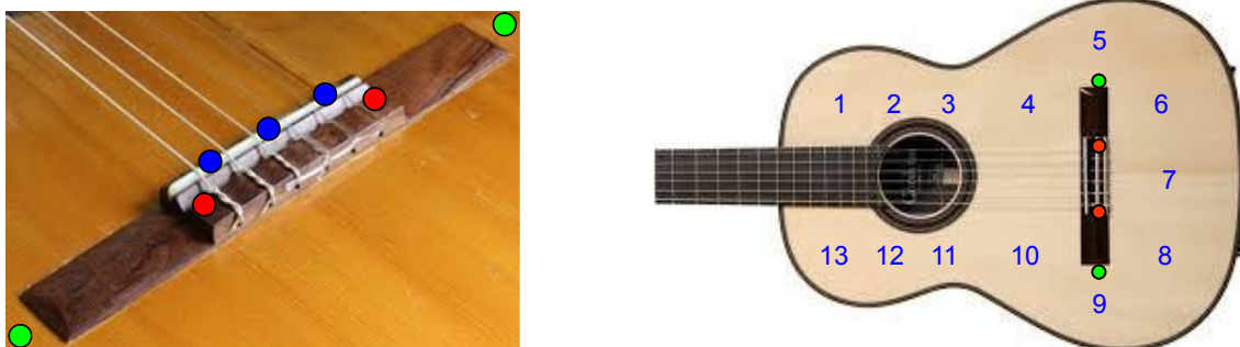
Figure 1. Setup with positions for hammer excitation (blue), acceleration sensors (red), and microphones (10 cm above green marks), for structural and radiation response from the bridge (left) and for temporal responses of the top (right).
