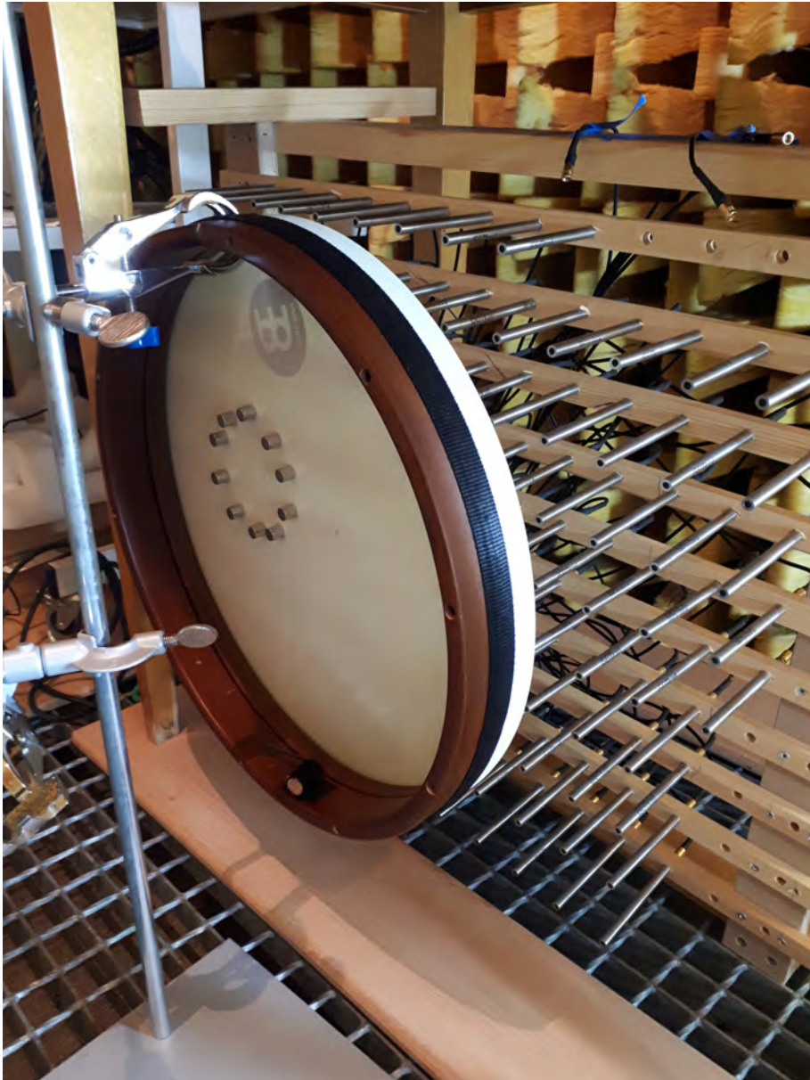
Figure 4. Modified frame drum positioned in front of the microphone array.
