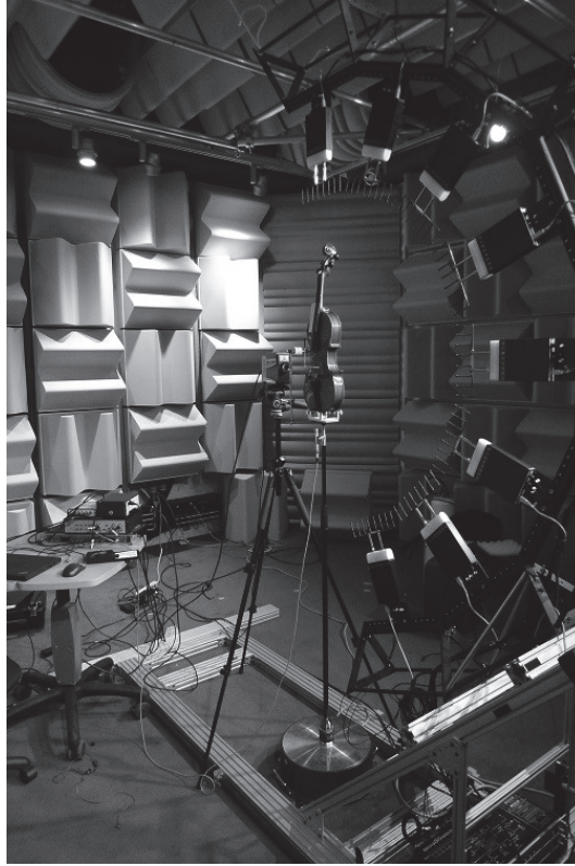
Figure 1. Semi-circular microphone array, rotating base, and support rig used to measure sound pressure signals at 4320 points on a one-meter-radius sphere around the violin. The laser Doppler vibrometer (on the tripod) was only used not used during the sound pressure measurements.
