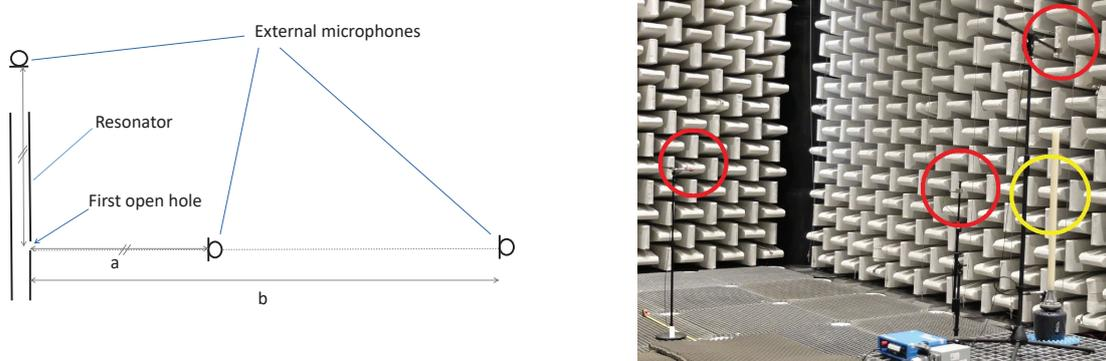
Figure 1. Three microphones (right, in red) are positioned around the resonator. The first two microphones are at the level of the first open hole (right, in yellow) and at a distance of  $b = 4$  m and  $a = 0.7$  m, respectively. The third is positioned above the end of the resonator at a distance  $a = 0.7$  m from the first open hole.
