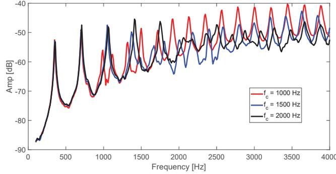
Figure 2. Transfer function between internal pressure and external pressure at the overhead microphone location. The resonators with  $f_c = 1000$ ,  $1500$ , and  $2000$  Hz are shown in red, blue, and black, respectively.
