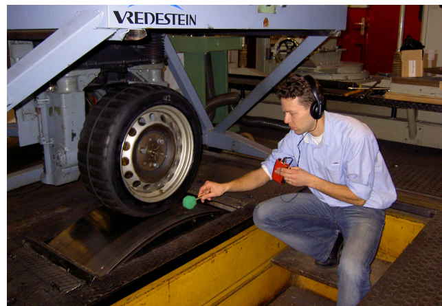
Figure 2: Tire -drum measurement set-up.
