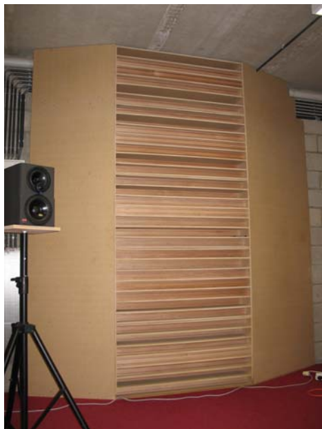
Figure 3: Diffusers placed on the rear wall.
