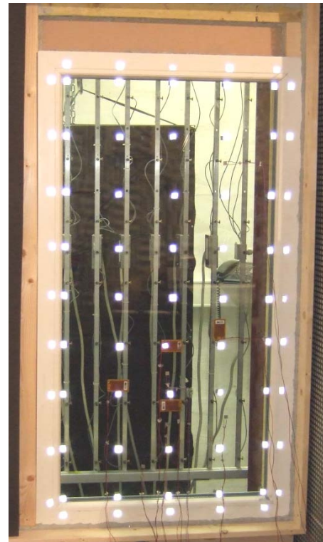
Figure 7: test stand for the active window: piezoelectric patch actuators, microphone array, reflecting dots for laser vibrometer measurements, loudspeaker in the background.
