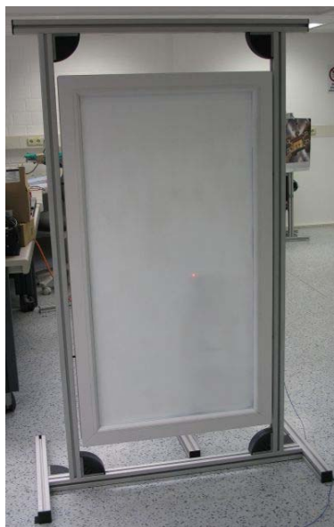
Figure 1: test stand with passive double-glazing window (red dot marks laser spot).
