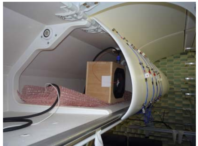
Figure 6: View into hat rack with custom built loudspeaker as sound source.
