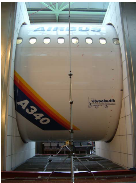
Figure 1: Test bed for acoustic ground tests (cross section of a long-range airliner)
