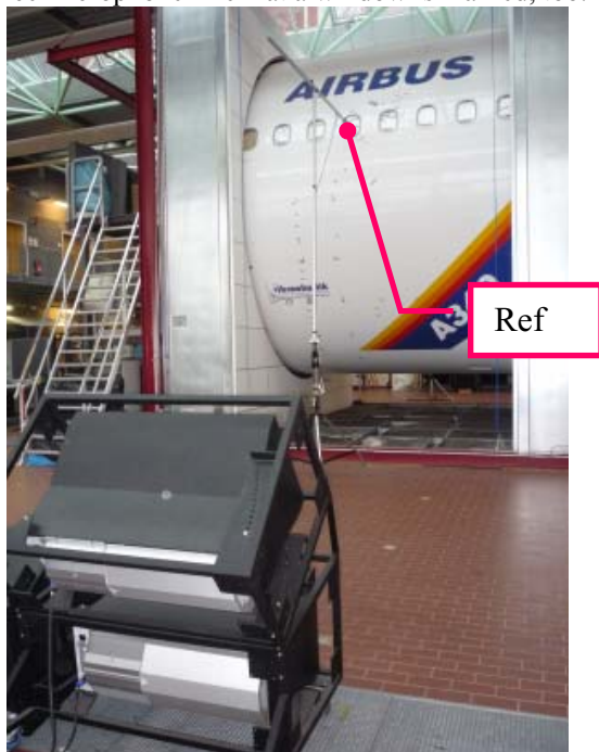
Figure 8: Set up for sound excitation with PA loudspeakers from the outside of the mock up.
