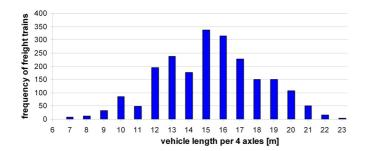
**Figure 1:** Distribution of average vehicle length of freight trains in the Netherlands. Lengths refer to 4 axles, so not necessarily from buffer to buffer.
