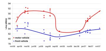
**Figure 3:** Long-term variations for the two outer vehicles of an EMU of type mDDM with serious wheel defects at the motor unit. After a maintenance action around September 2006 the problem occured again in February 2007. The measurements were taken at different sites and where not corrected for rail roughness differences.
