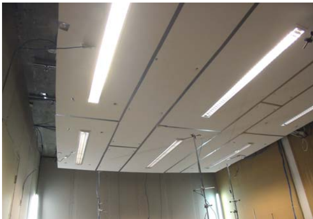
Figure 3: One of the investigated ceiling configurations in the climatic chamber consisting of 40 mm mineral wool.
