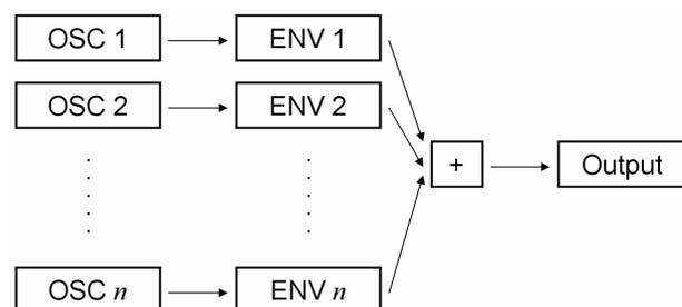
**Figure 1:** Principal block diagram of the synthesis algorithm. Freely programmable wavetable synthesizers are used.
