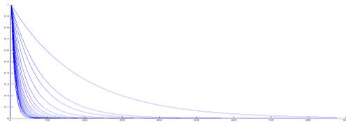
**Figure 2:** Example of a series of amplitude envelopes. The envelope on top is the fitted model of the decay time. All curves below show faster decays due to high-frequency damping.
