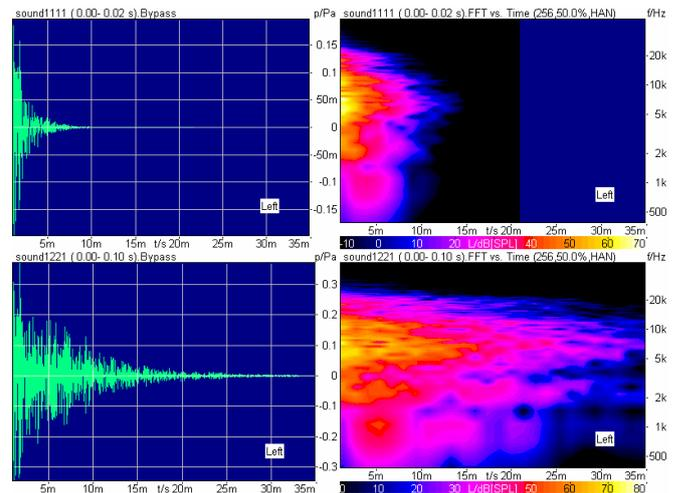
**Figure 3:** Two examples of synthesized stimuli. The upper signal uses fast attack and decay settings, the lower signal uses slow settings. Spectral composition and damping are the same for both stimuli.
