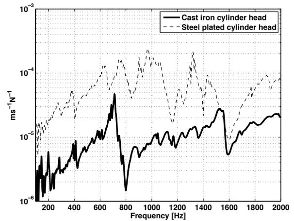
Figure 10: Driving point mobility prototype and redesigned cylinder head.
