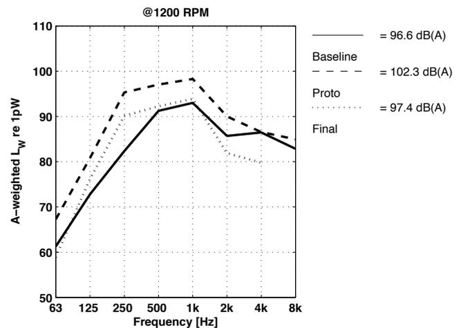
Figure 11: Compressor sound power level of Grasso 412 (baseline), prototype Grasso V700 (proto) and pre-production Grasso V700 (final).
