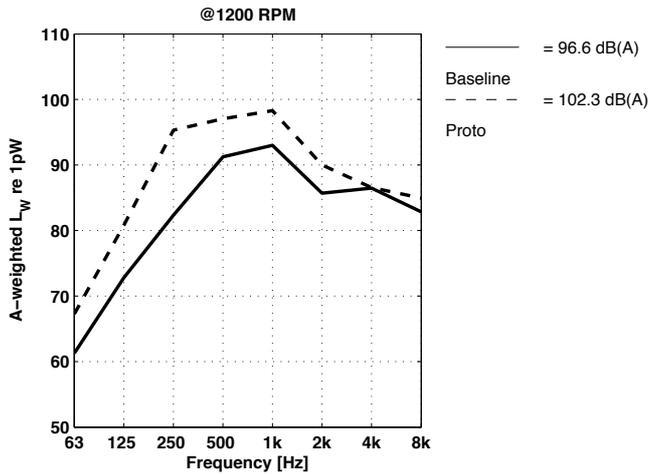
**Figure 3:** A-weighted Soundpower Spectrum of Grasso 412 (baseline) and prototype Grasso V700 (proto).
