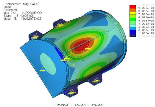
**Figure 6:** Predicted natural mode at approximately 1000 Hz, Grasso V700 prototype
