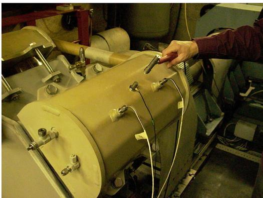
**Figure 4:** Cylinder head driving point measurement set-up. The driving point measurements were performed using a hammer, which was instrumented with a Apteck force transducer, type AU-01. A Bruel&Kjaer accelerometer type 4383 was placed nearby the point of excitation to measure the structural response due to the hammer excitation.
