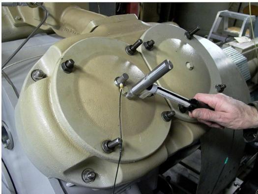
Figure 9: Ductile cast iron cylinder head driving point measurement set-up.
