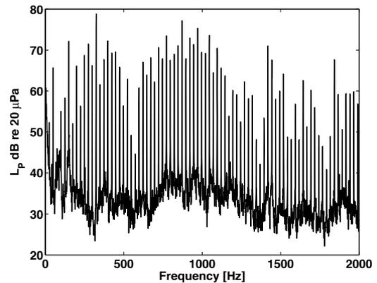
Figure 2: Typical sound pressure level, compressor operating at 1200 rpm.
