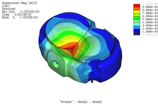
Figure 8: Ductile cast iron cylinder head predicted normal mode at 1320 Hz.
