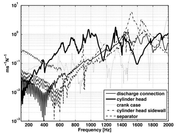
**Figure 5:** Structural mobility measurements taken on a number of plate-like structural parts of the compressor.
