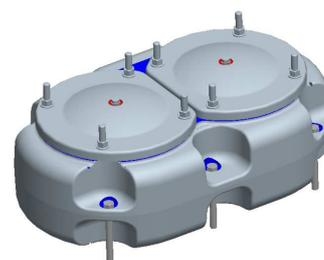
**Figure 7:** Solid model of the ductile cast iron cylinder head
