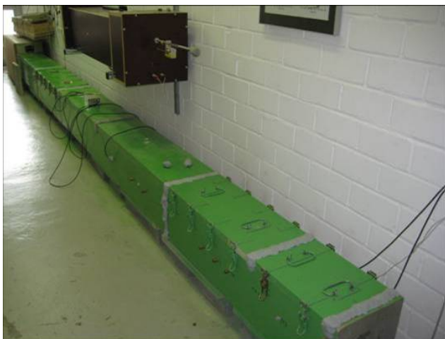
Figure 1: Standing wave tube used in first measurements.
