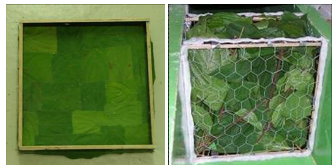
Figure 2: Probes for standing wave tube. a) sheet made by leaves glued together, b) probe of plant material in a lattice box.
