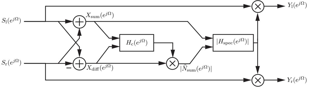
**Figure 1:** Block diagram of the binaural spectral subtraction beamformer algorithm. The binaural microphone signals are filtered with an compensation filter by using the spectral subtraction. Interaural level and time differences will be preserved.
