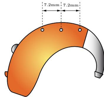
**Figure 2:** for the evaluation used hearing aid dummy, containing a receiver and three microphones in a distance of 7.2mm
