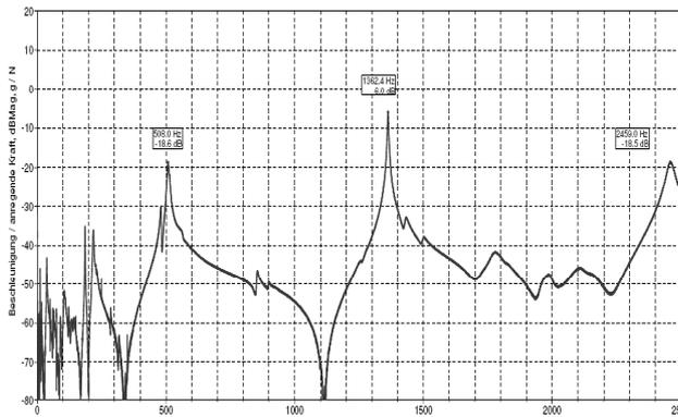
**Figure 7:** the wheel’s transfer function at test stand (wheel for operator B) original damper with impurities painted on contact surface (see no. 3 in table 1)
