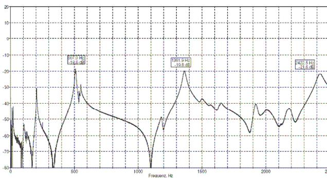
**Figure 8:** the wheel’s transfer function at test stand (wheel for operator B) with new developed damper with impurities painted on contact surface (see no. 7 in table 1)
