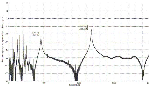
Figure 4: the wheel's transfer function at the vehicle (operator A) before reassembling. Maximal peak level of mode(3,0) resonance is -13.3 dB.
