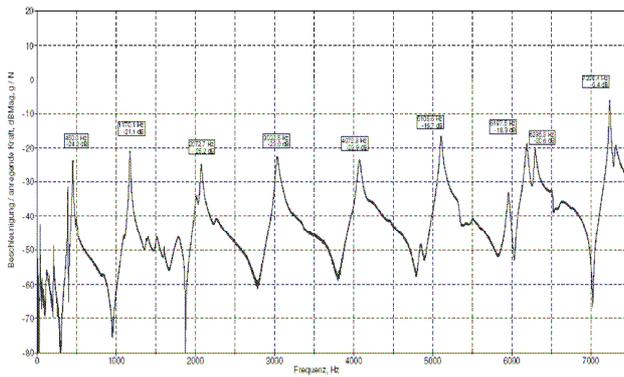
Figure 3: transfer function damped wheel operator A
