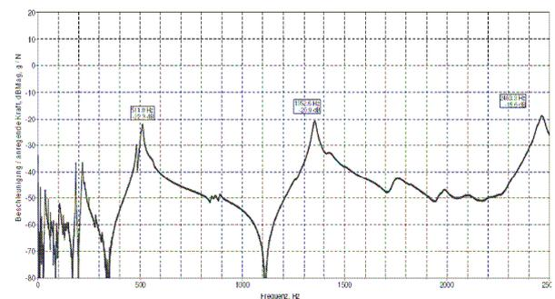
Figure 6: the wheel's transfer function at test stand (wheel for operator B) original damper (see no. 2 in table 1)
