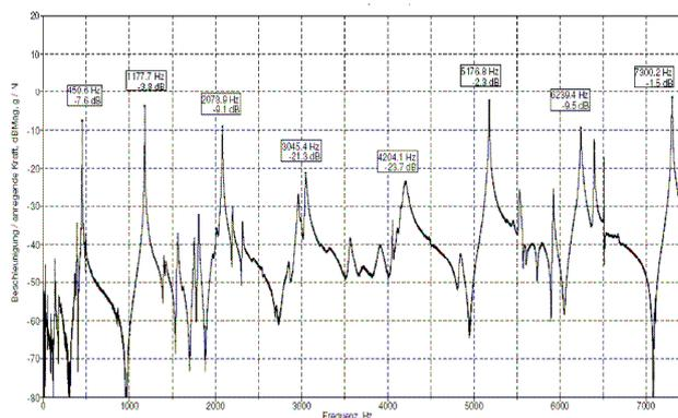
Figure 2: transfer function undamped wheel operator A
