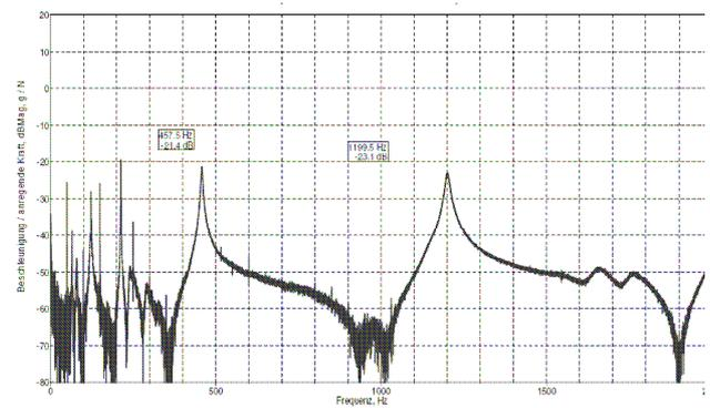
Figure 5: transfer function measured after cleaning the contact surface of the wheel, measured at vehicle of operator A. Maximal peak level of mode(3,0) resonance is -23.1 dB.
